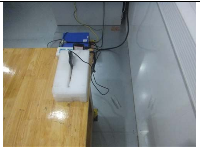
Conducted Emissions Test Setup Side View
