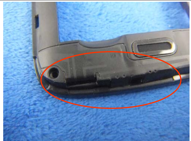
GSM/PCS/UMTS-FDD Antenna View
