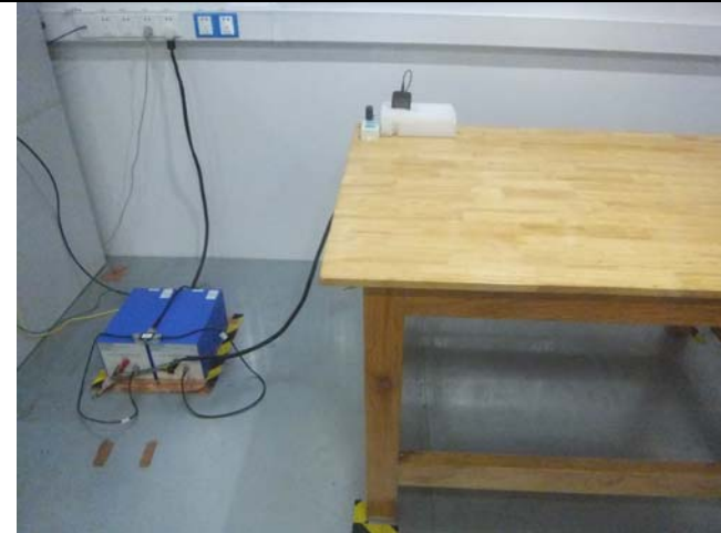
Conducted Emissions Test Setup Front View
