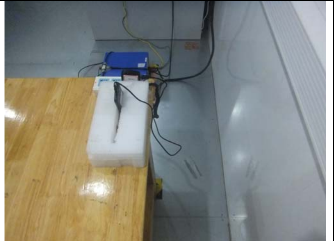
Conducted Emissions Test Setup Side View
