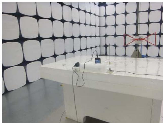
Radiated Spurious Emissions Test Setup Below 1GHz
