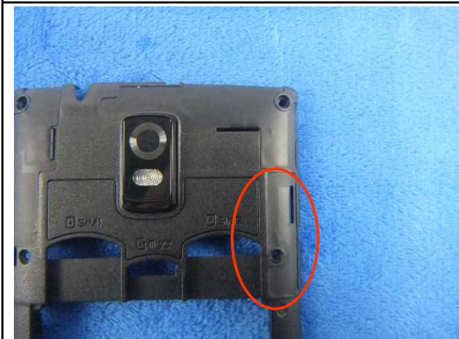
BT/WIFI Antenna View
