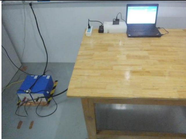
Conducted Emissions Test Setup – Front View
