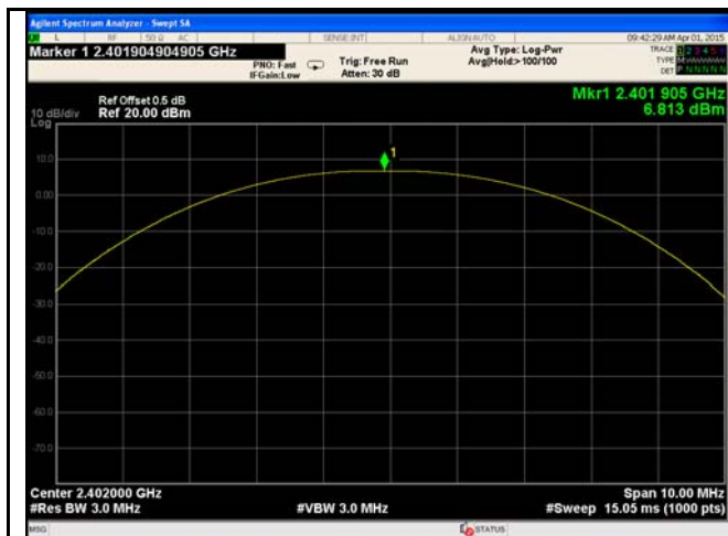
GFSK Output power - Low CH 2402
