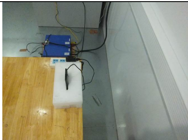
Conducted Emissions Test Setup Side View
