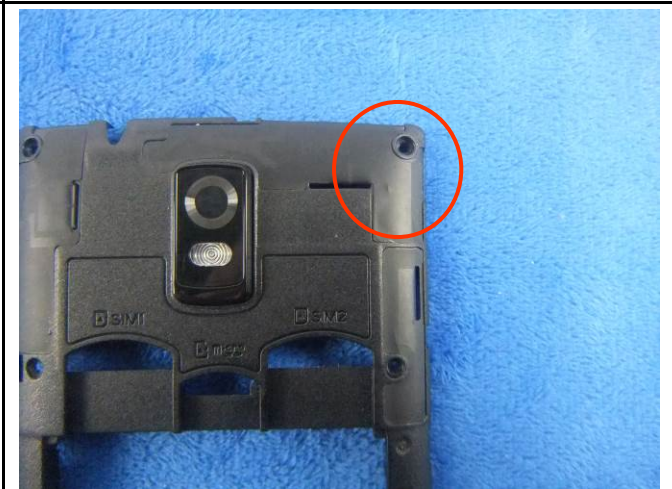
GSM/PCS/UMTS/-FDD Antenna View
