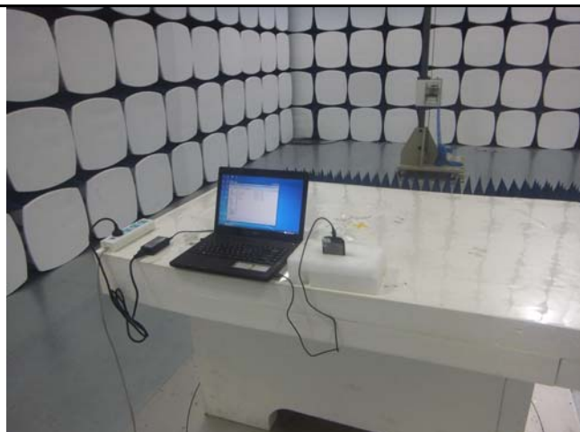
Radiated Spurious Emissions Test Setup Above 1GHz
