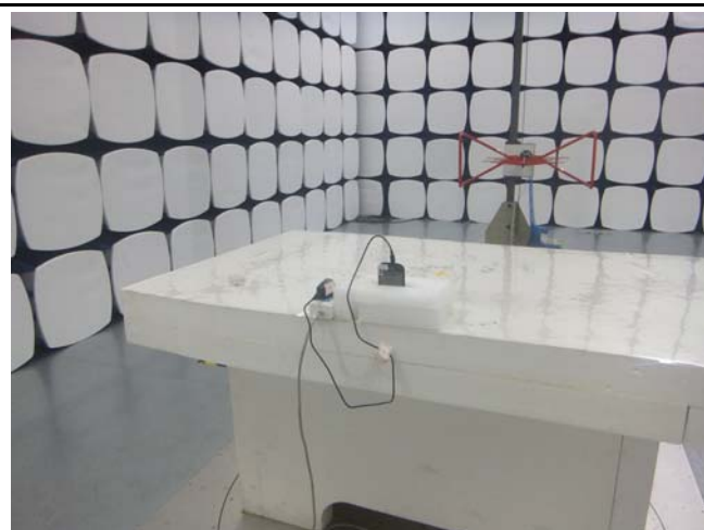
Conducted Emissions Test Setup Front View
