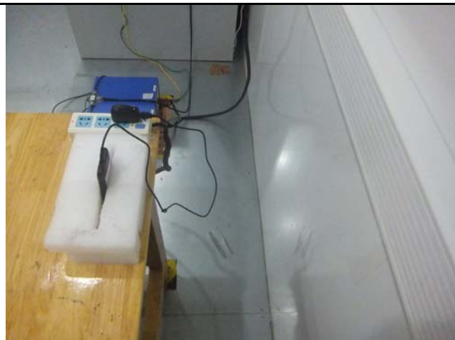
Conducted Emissions Test Setup Side View
