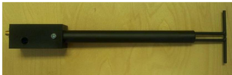
Figure 1 – MVG COMOSAR Validation Dipole
