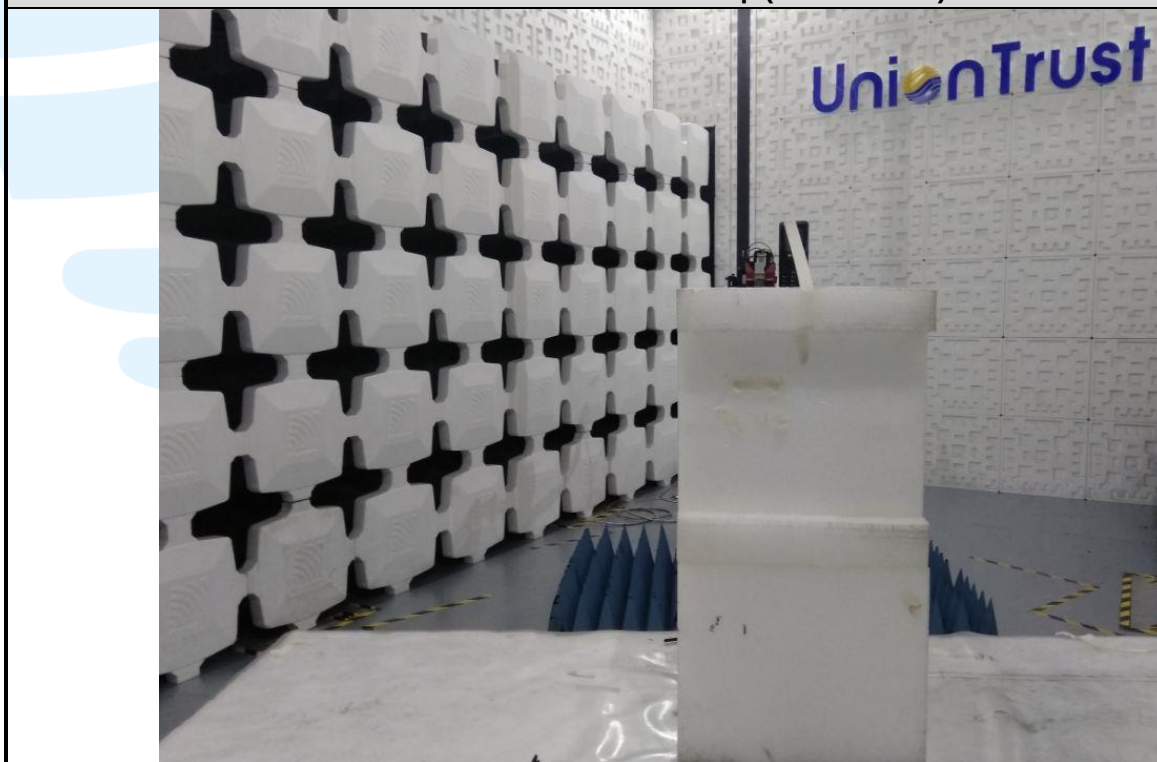
Radiated emission Test Setup (Above 1 GHz)
