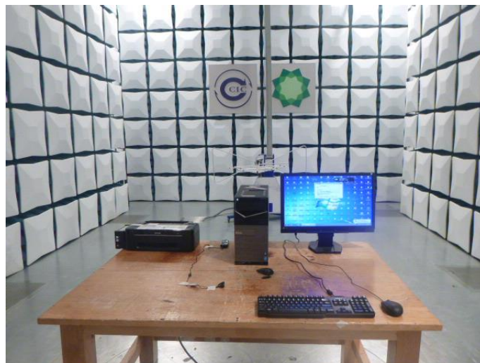
Radiated Emission (above 1GHz) Connect to PC
