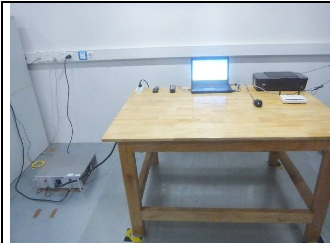
Conducted Emissions Test Setup – Front View
