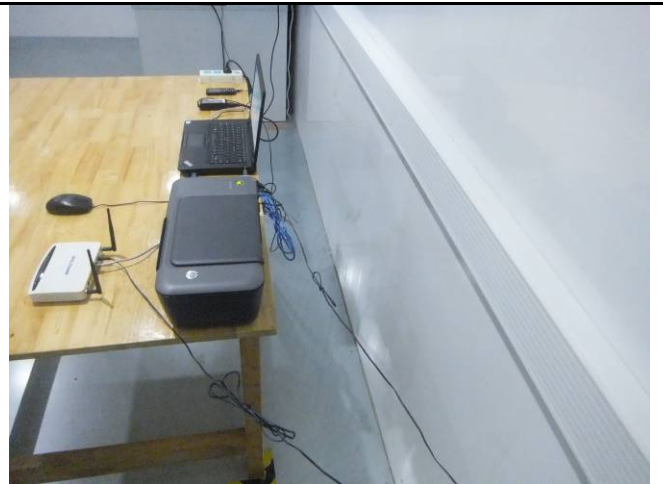
Conducted Emissions Test Setup – Side View
