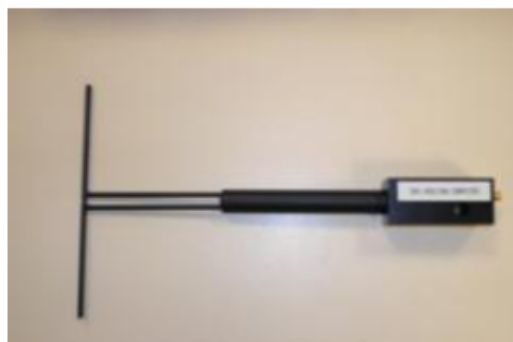
Figure 1 – Satimo COMOSAR Validation Dipole
