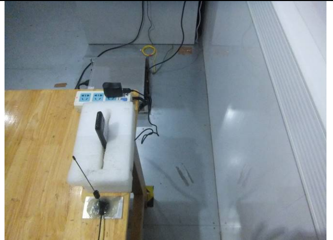
Conducted Emissions Test Setup Side View
