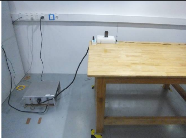
Conducted Emissions Test Setup Front View
