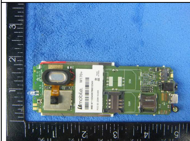
Mainboard with Shielding - Front View
