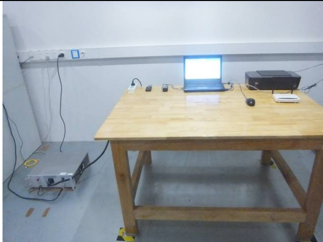
Conducted Emissions Test Setup – Front View
