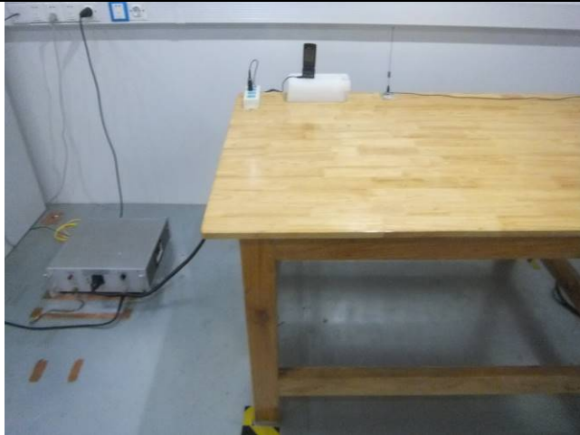
Conducted Emissions Test Setup Front View
