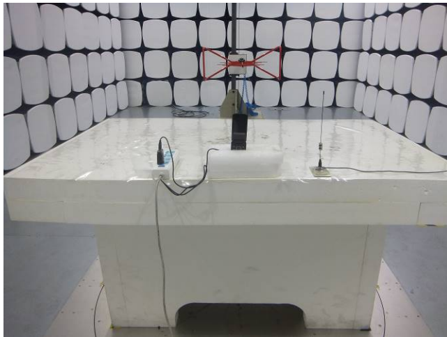
Radiated Spurious Emissions Test Setup Below 1GHz
