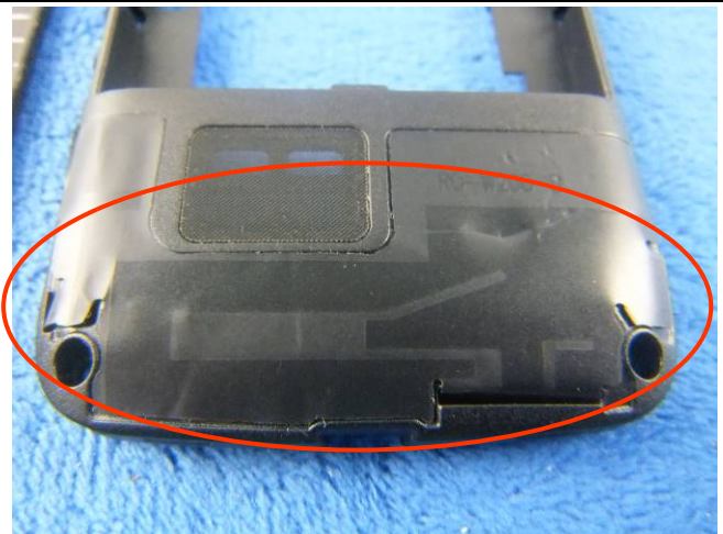
GSM/PCS/UMTS-FDD Antenna View
