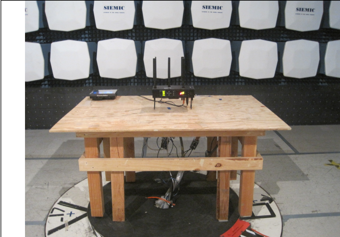
Radiated Emission Test Setup – Front View
