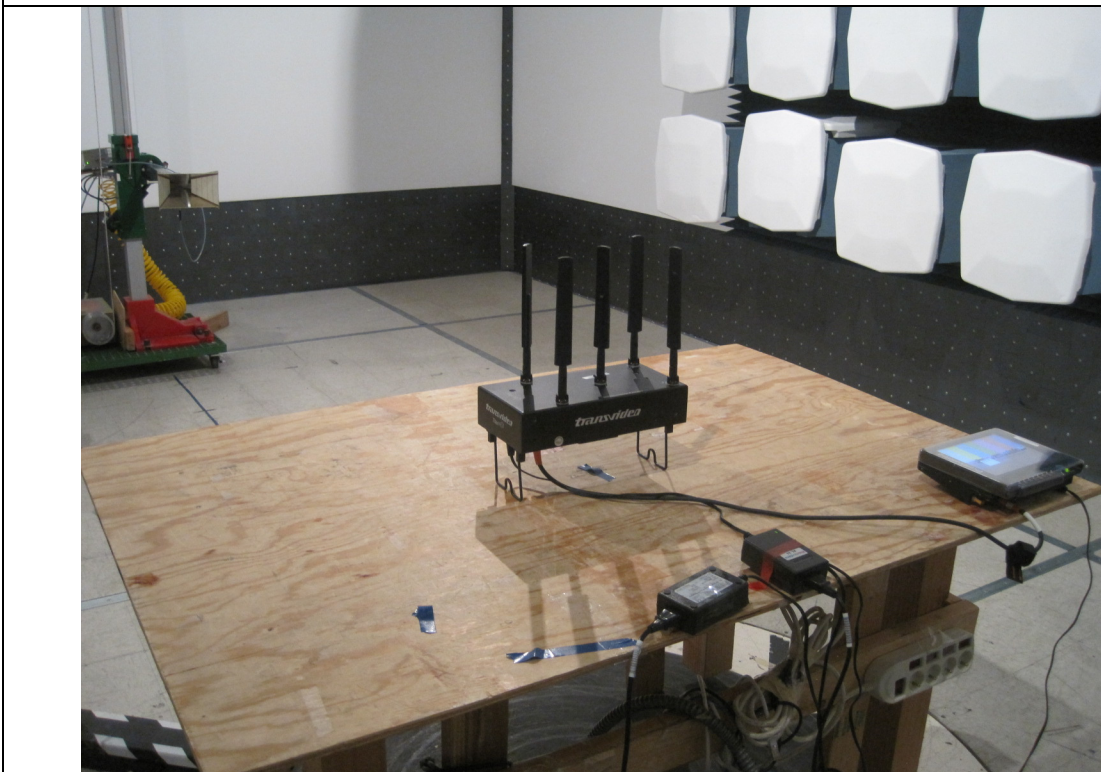
Radiated Emission Test Setup – Rear View
