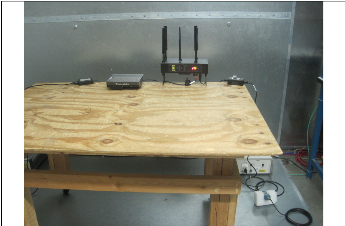
Radiated Emission Test Setup – Front View
