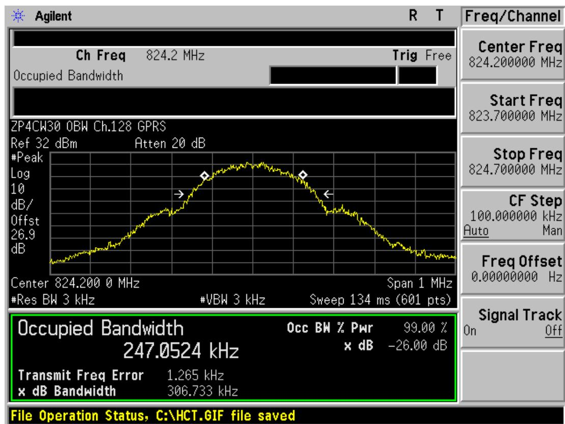
■ GSM850 MODE (190 CH.) Occupied Bandwidth
