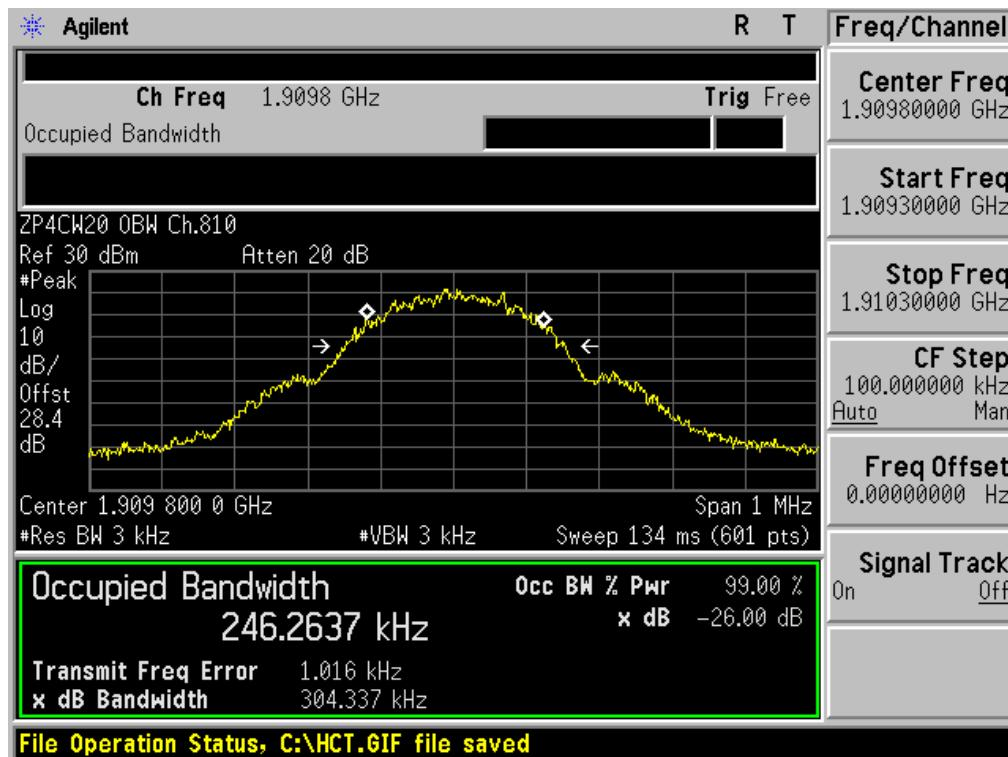
■ GSM1900 EDGE (512 CH.) Occupied Bandwidth
