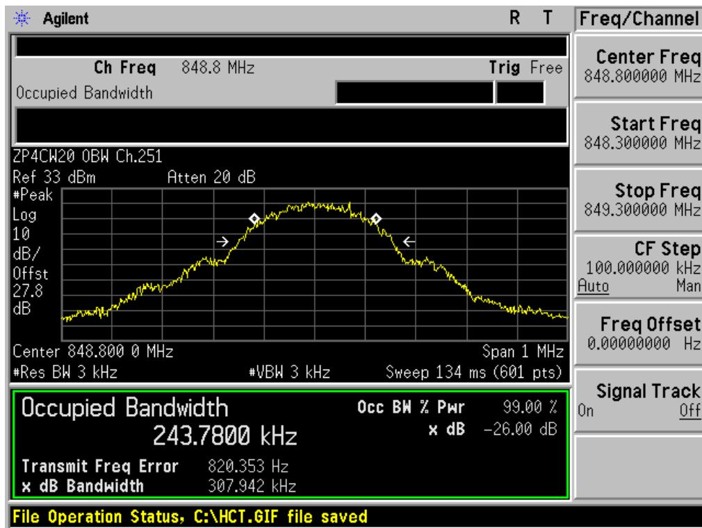
■ GSM850 EDGE (190 CH.) Occupied Bandwidth
