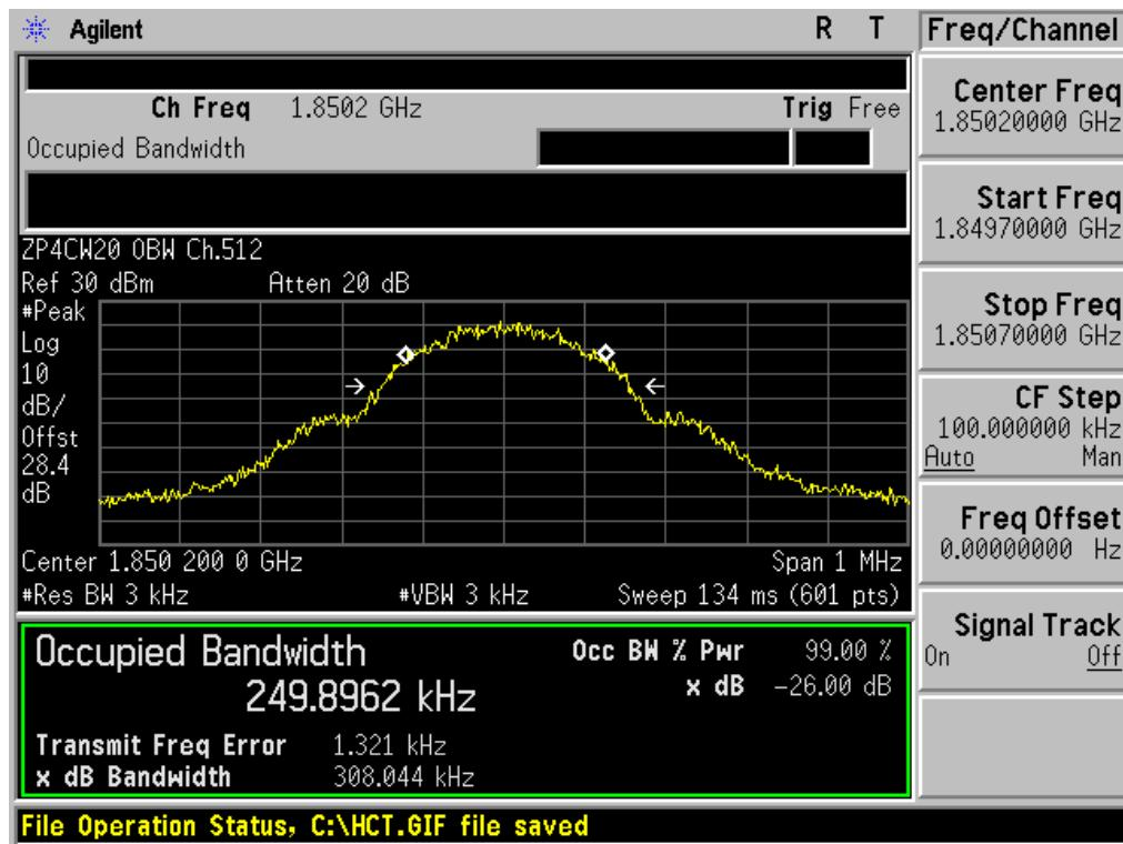
■ GSM1900 MODE (661 CH.) Occupied Bandwidth
