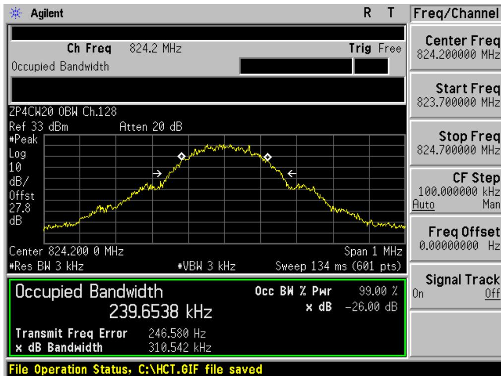
■ GSM850 MODE (190 CH.) Occupied Bandwidth
