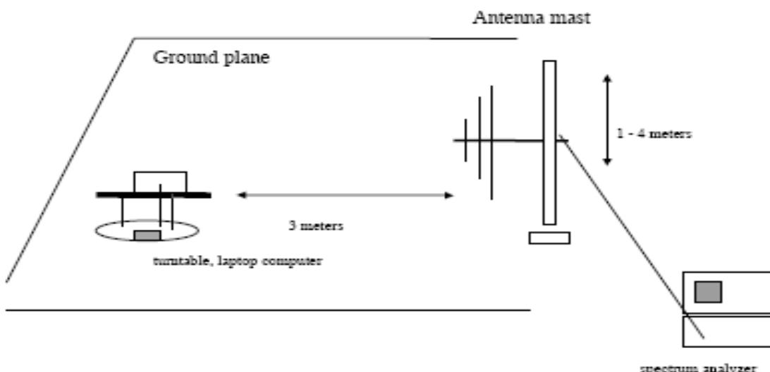
Test Procedures: Radiated emissions were measured according to ANSI C63.4.
