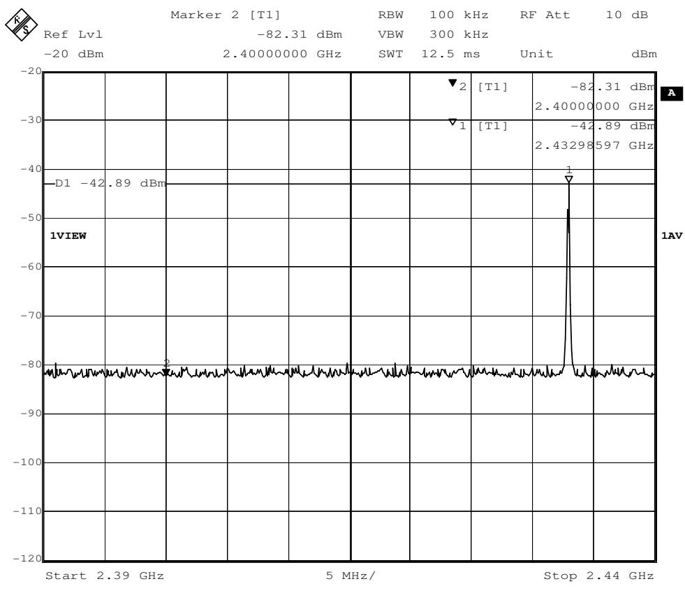
For 2.40 GHz band edge checked with 2.433 GHz frequency operated, the delta shown at the plots are -39.30 dB for peak detector mode and -39.42 dB for Average detector mode.
