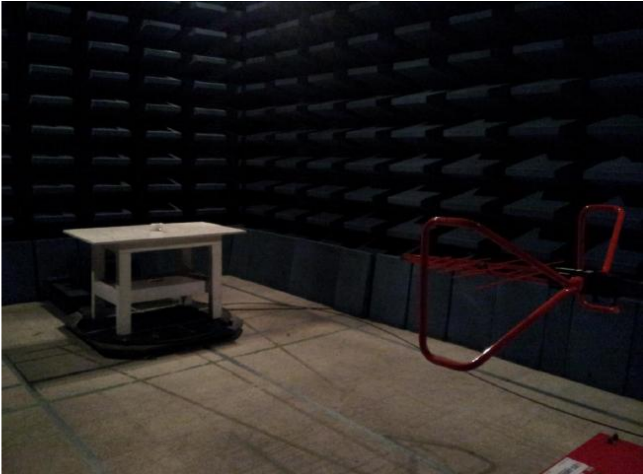
Radiated Emissions Test-Setup 30MHz-1GHz
