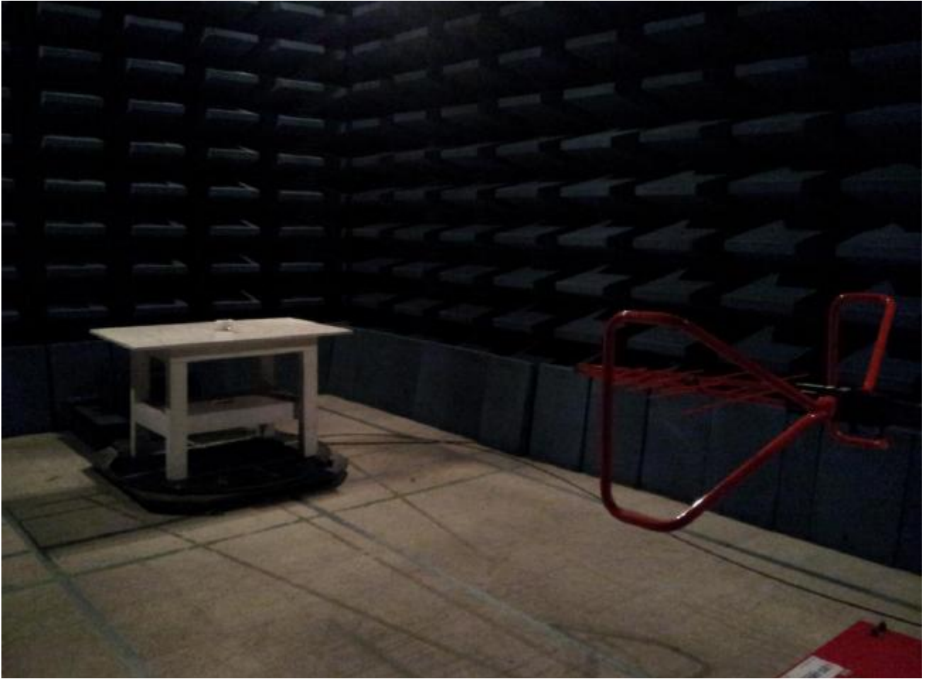
Radiated Emissions Test-Setup 30MHz-1GHz
