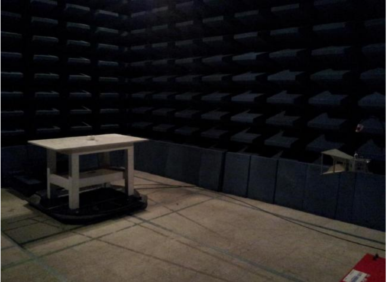
Radiated Emissions Test-Setup above 1GHz
