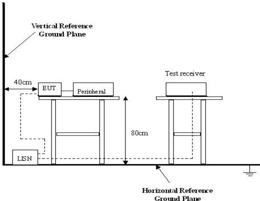
The EUT was placed on the test table in ON mode.
