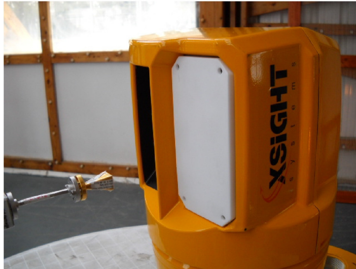
Photograph 7.3.2 Setup for radiated emissions measurements above 40 GHz, EUT close view
