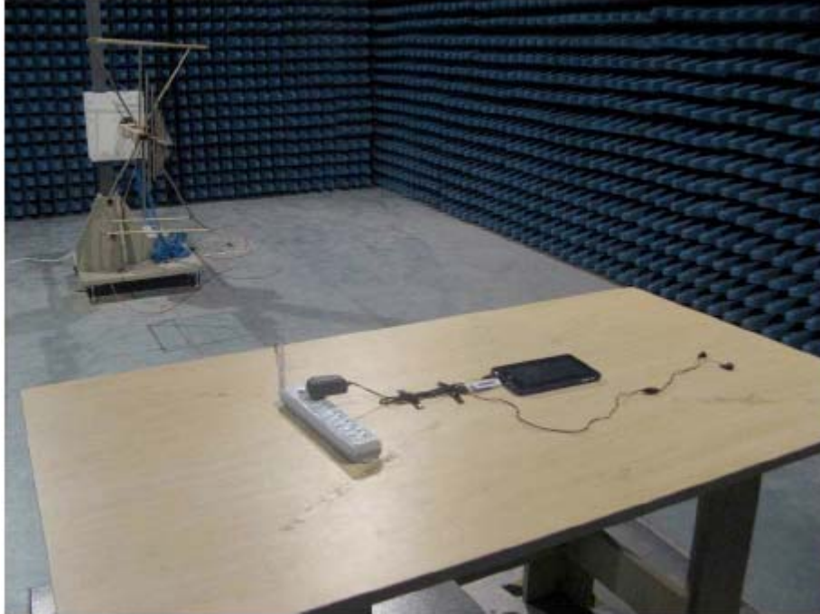
RADIATED EMISSION TEST SETUP
