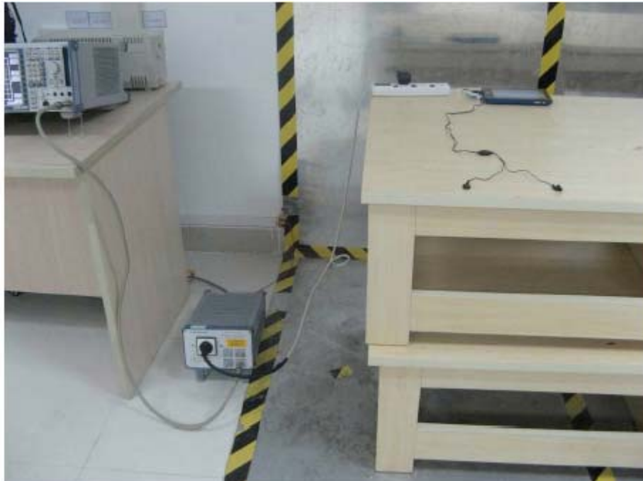
CONDUCTED EMISSION TEST SETUP
