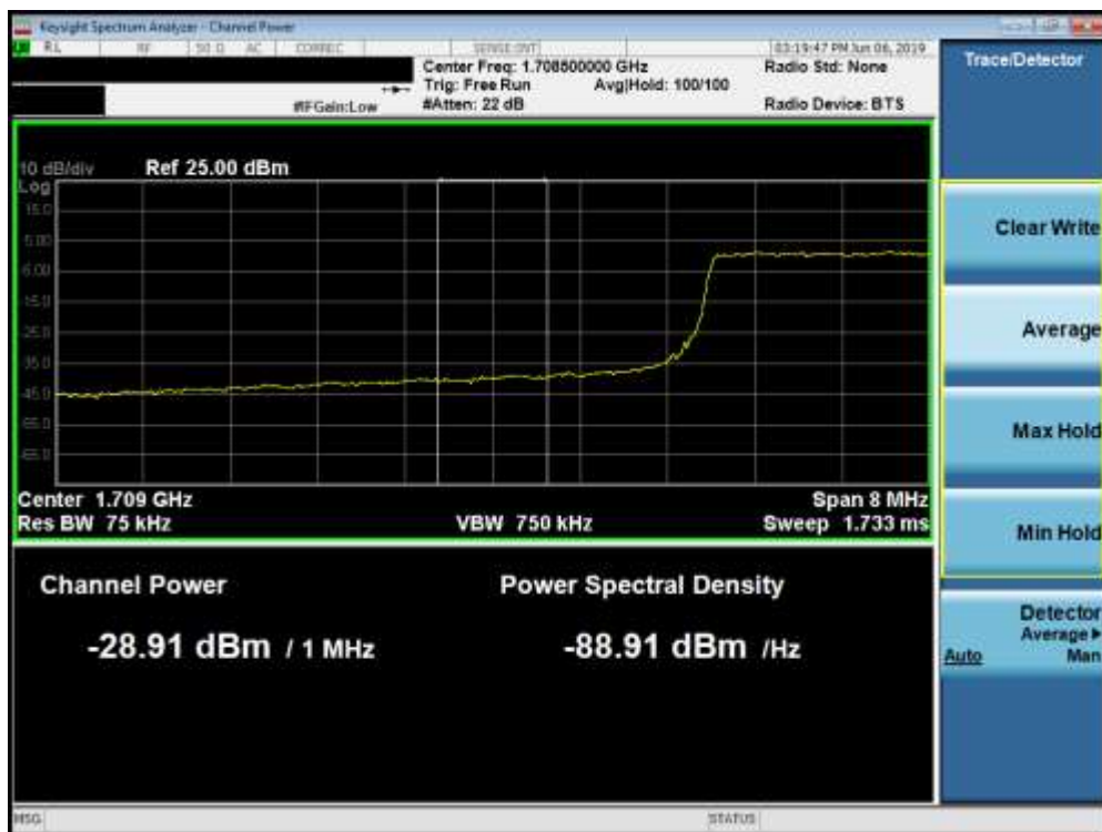
Plot 7-146. Lower Extended Band Edge Plot (Band 66/4 - 10.0MHz QPSK - Full RB Configuration)
