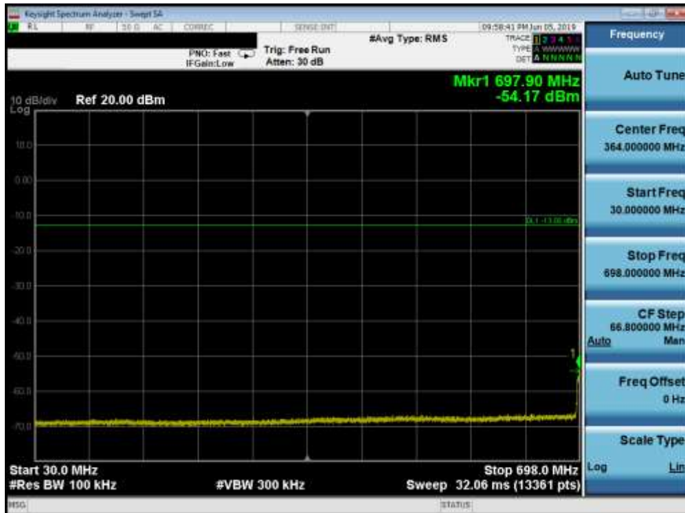
Plot 7-56. Conducted Spurious Plot (Band 12/17 - 10.0MHz QPSK - RB Size 1, RB Offset 0 - Mid Channel)
