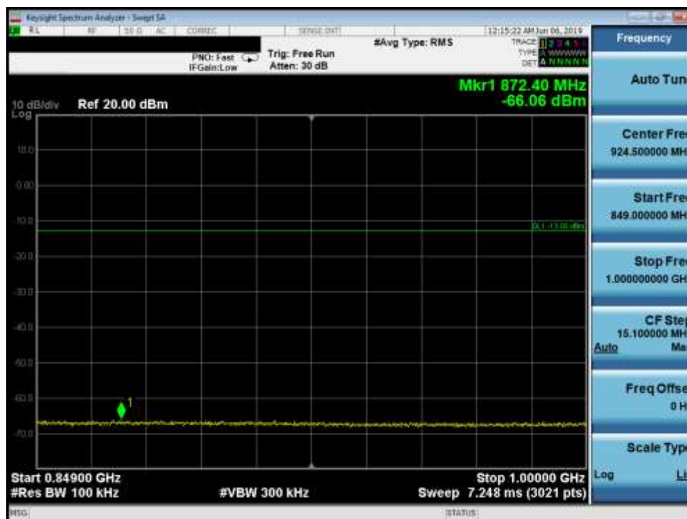
Plot 7-66. Conducted Spurious Plot (Band 5 - 10.0MHz QPSK - RB Size 1, RB Offset 0 - Low Channel)
