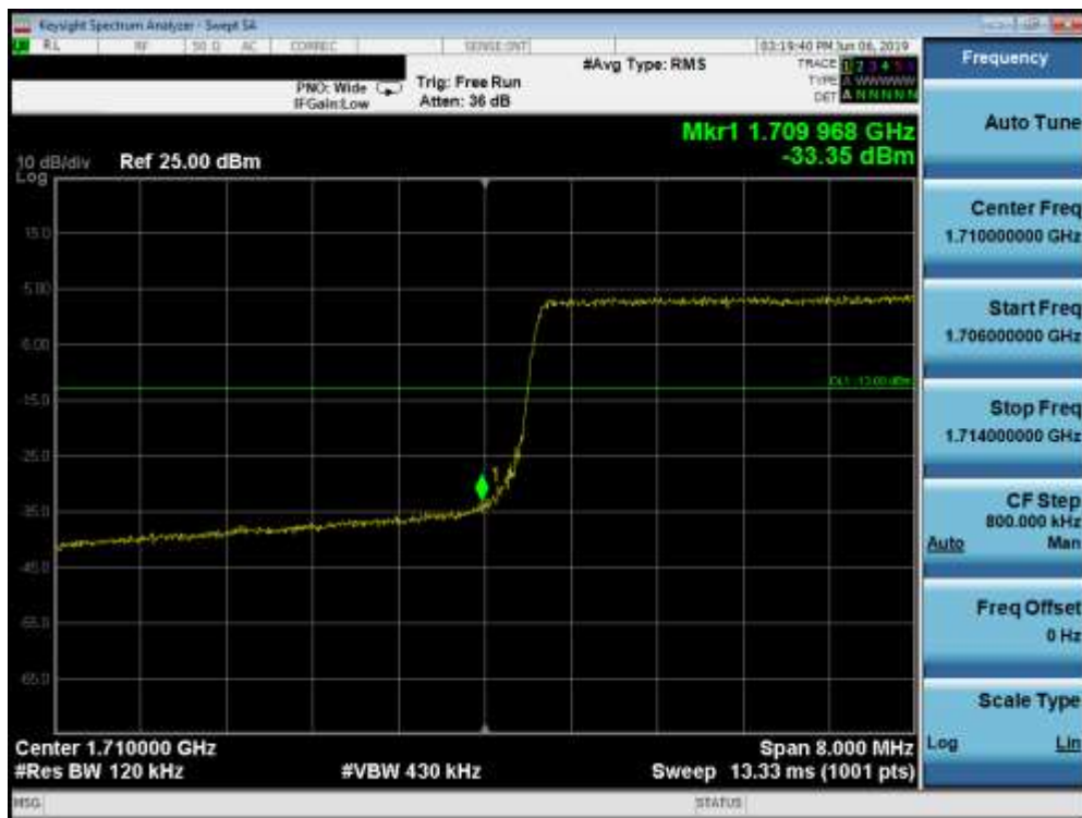
Plot 7-145. Lower Band Edge Plot (Band 66/4 - 10.0MHz QPSK - Full RB Configuration)
