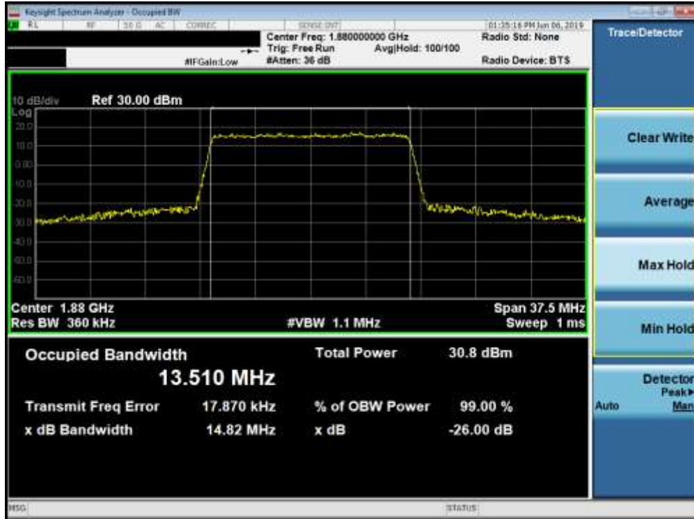
Plot 7-41. Occupied Bandwidth Plot (Band 2 - 15.0MHz QPSK - Full RB Configuration)
