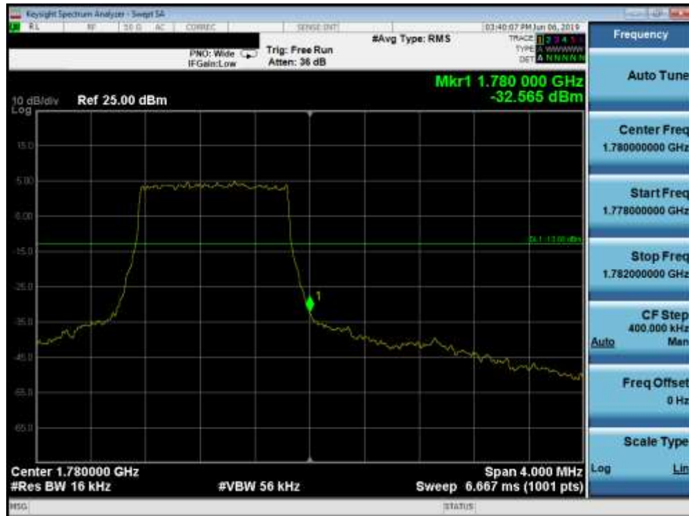
Plot 7-131. Upper Band Edge Plot (Band 66 - 1.4MHz QPSK - Full RB Configuration)
