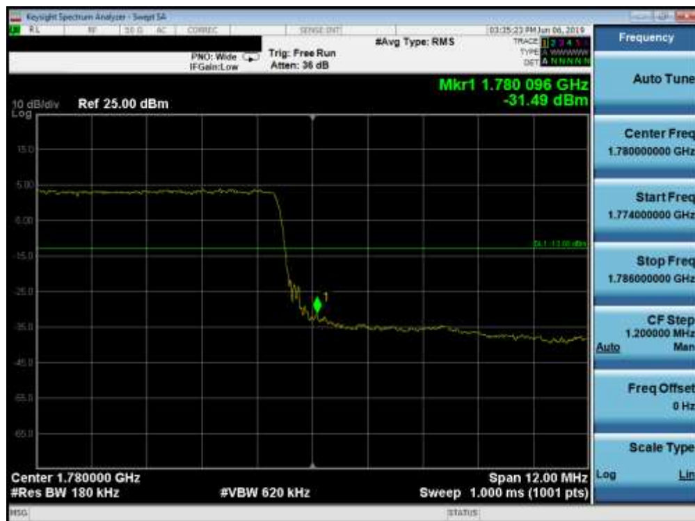
Plot 7-155. Upper Band Edge Plot (Band 66 - 15.0MHz QPSK - Full RB Configuration)
