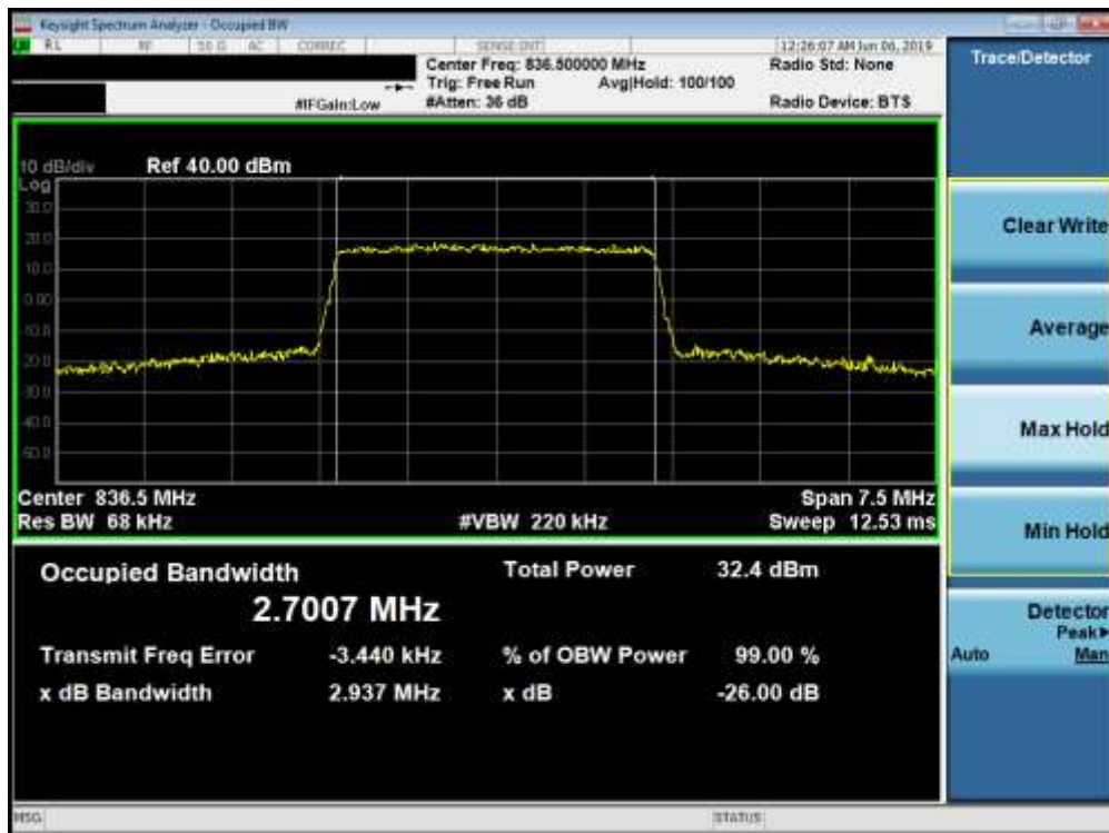
Plot 7-15. Occupied Bandwidth Plot (Band 5 - 3.0MHz QPSK - Full RB Configuration)
