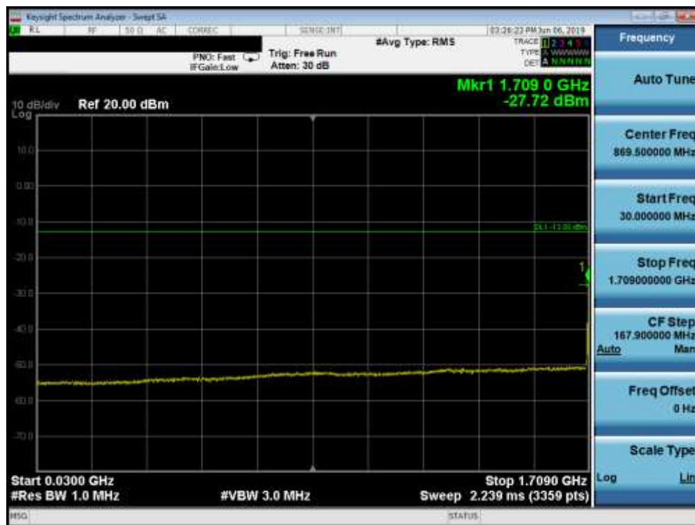
Plot 7-74. Conducted Spurious Plot (Band 66/4 - 20.0MHz QPSK - RB Size 1, RB Offset 0 - Low Channel)
