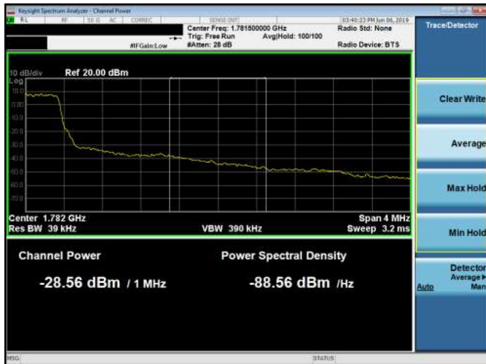
Plot 7-132. Upper Extended Band Edge Plot (Band 66 - 1.4MHz QPSK - Full RB Configuration)
