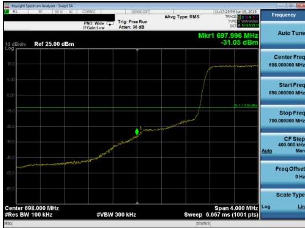
Plot 7-101. Lower Band Edge Plot (Band 12 - 1.4MHz QPSK - Full RB Configuration)
