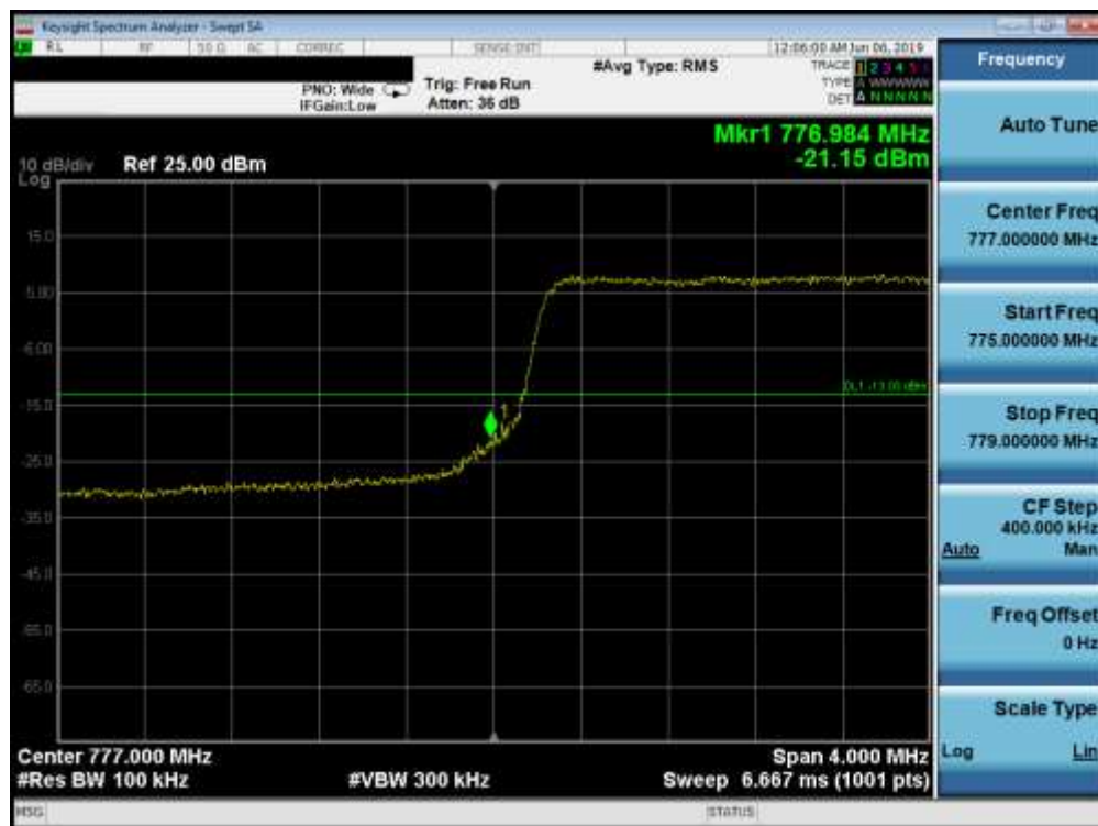
Plot 7-111. Lower Band Edge Plot (Band 13 - 5.0MHz QPSK - Full RB Configuration)
