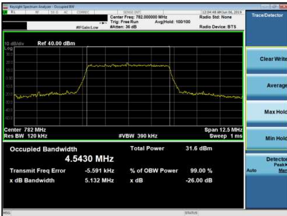
Plot 7-10. Occupied Bandwidth Plot (Band 13 - 5.0MHz 16-QAM - Full RB Configuration)
