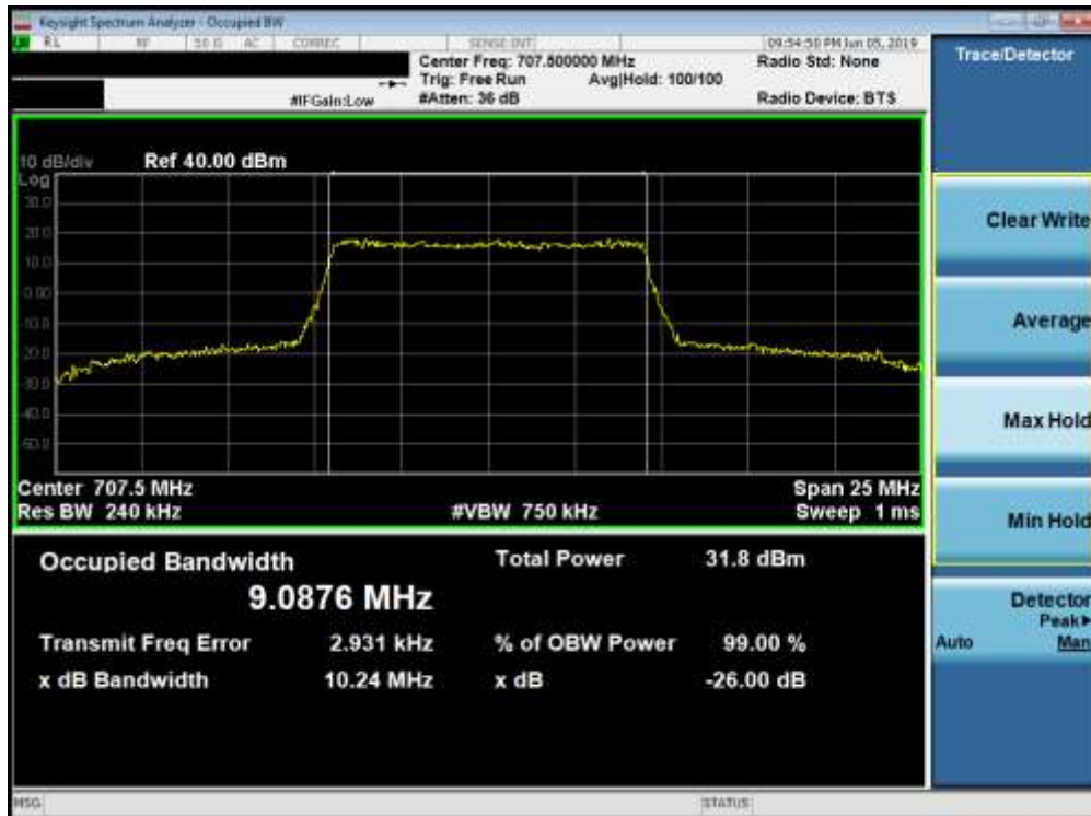
Plot 7-8. Occupied Bandwidth Plot (Band 12/17 - 10.0MHz 16-QAM - Full RB Configuration)
