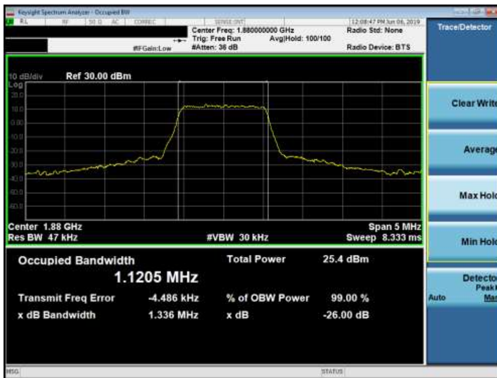
Plot 7-33. Occupied Bandwidth Plot (Band 2 - 1.4MHz QPSK - Full RB Configuration)
