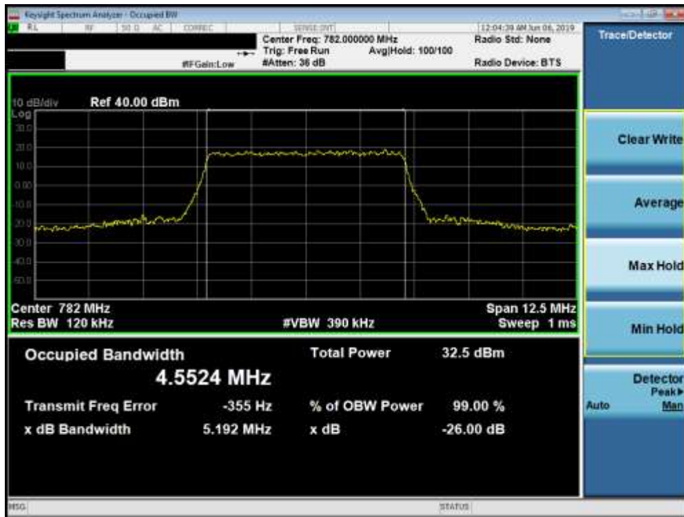
Plot 7-9. Occupied Bandwidth Plot (Band 13 - 5.0MHz QPSK - Full RB Configuration)
