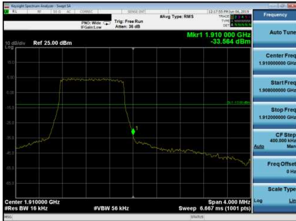
Plot 7-165. Upper Band Edge Plot (Band 2 - 1.4MHz QPSK - Full RB Configuration)
