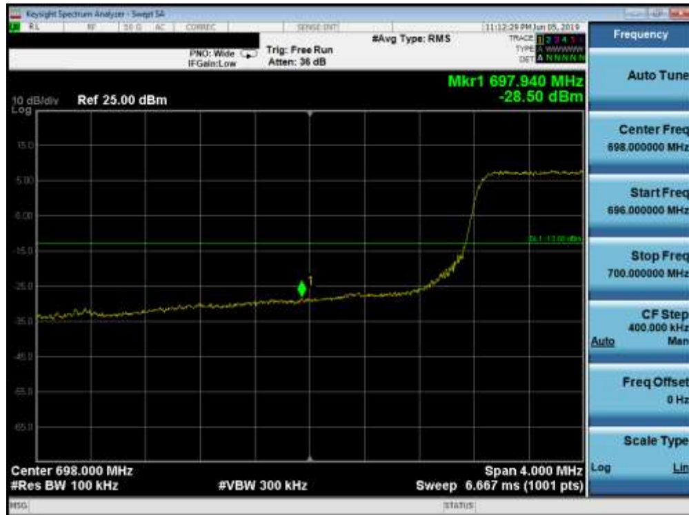
Plot 7-105. Lower Band Edge Plot (Band 12 - 5.0MHz QPSK - Full RB Configuration)
