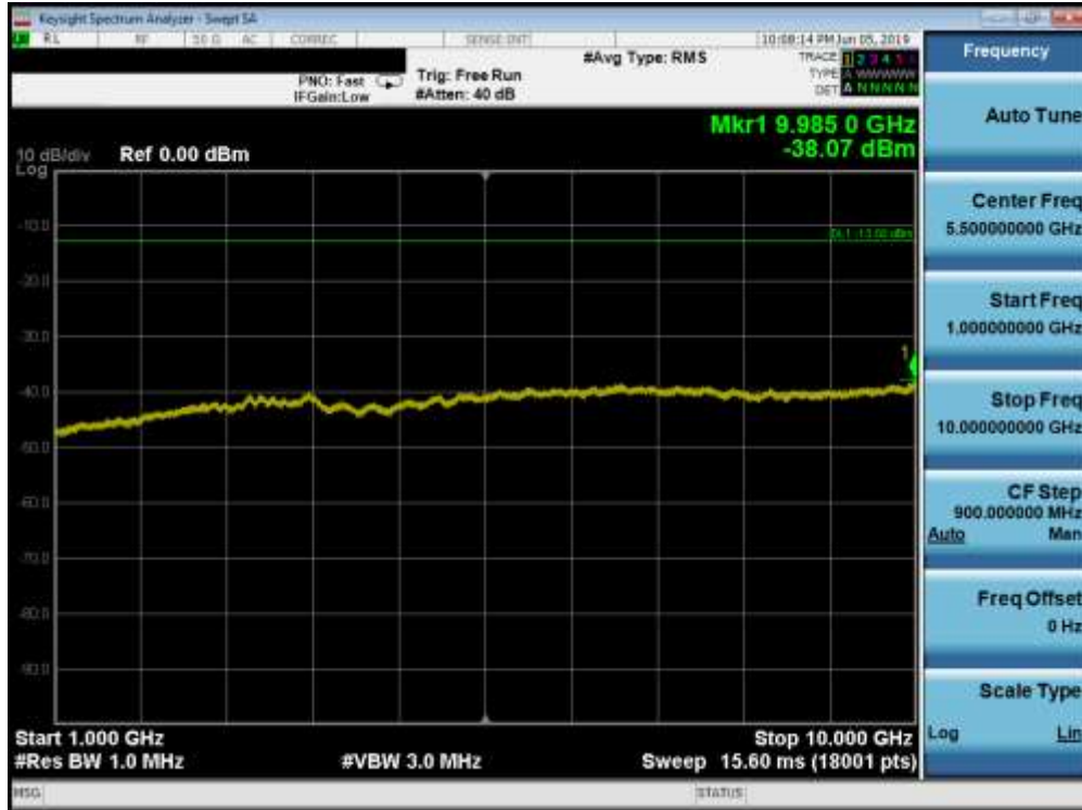
Plot 7-55. Conducted Spurious Plot (Band 12/17 - 10.0MHz QPSK - RB Size 1, RB Offset 0 - Low Channel)
