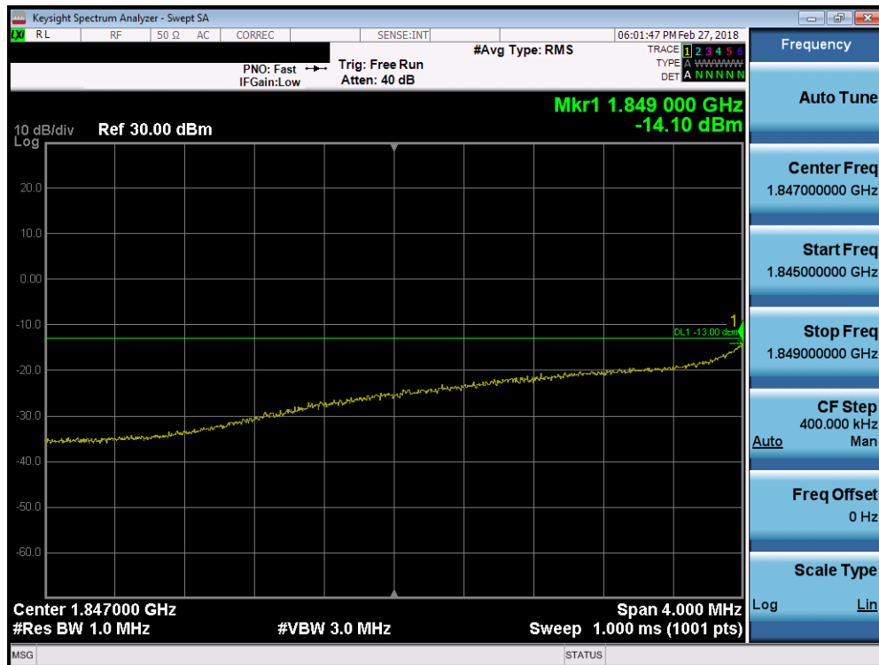
Plot 7-66. 4MHz Span Plot (PCS WCDMA Mode - Low Channel)
