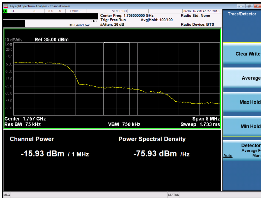
Plot 7-64. 4MHz Span Plot (AWS WCDMA Mode - High Channel)
