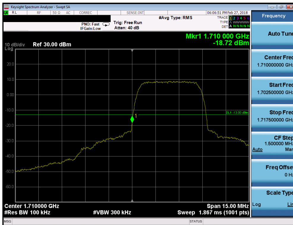
Plot 7-61. Band Edge Plot (AWS WCDMA Mode - Low Channel)
