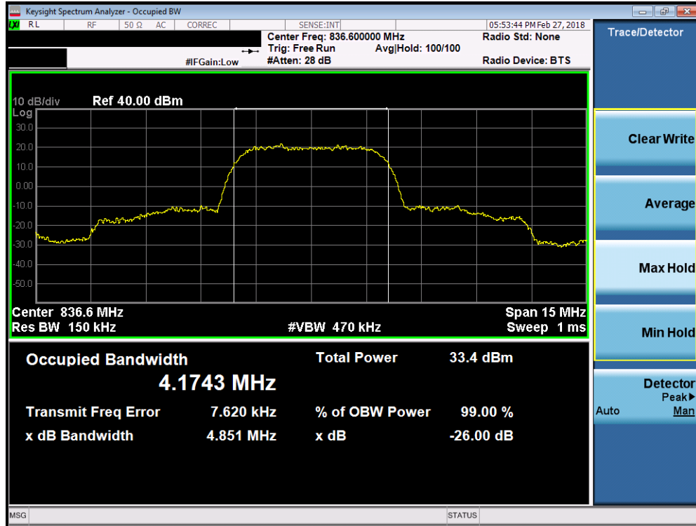
Plot 7-5. Occupied Bandwidth Plot (Cellular WCDMA Mode)
