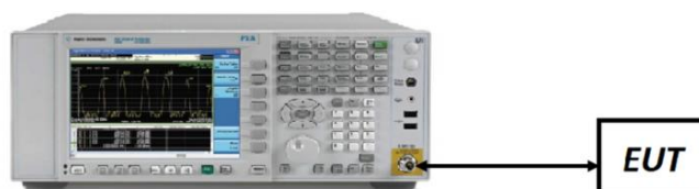
Figure 7-1. Test Instrument & Measurement Setup
