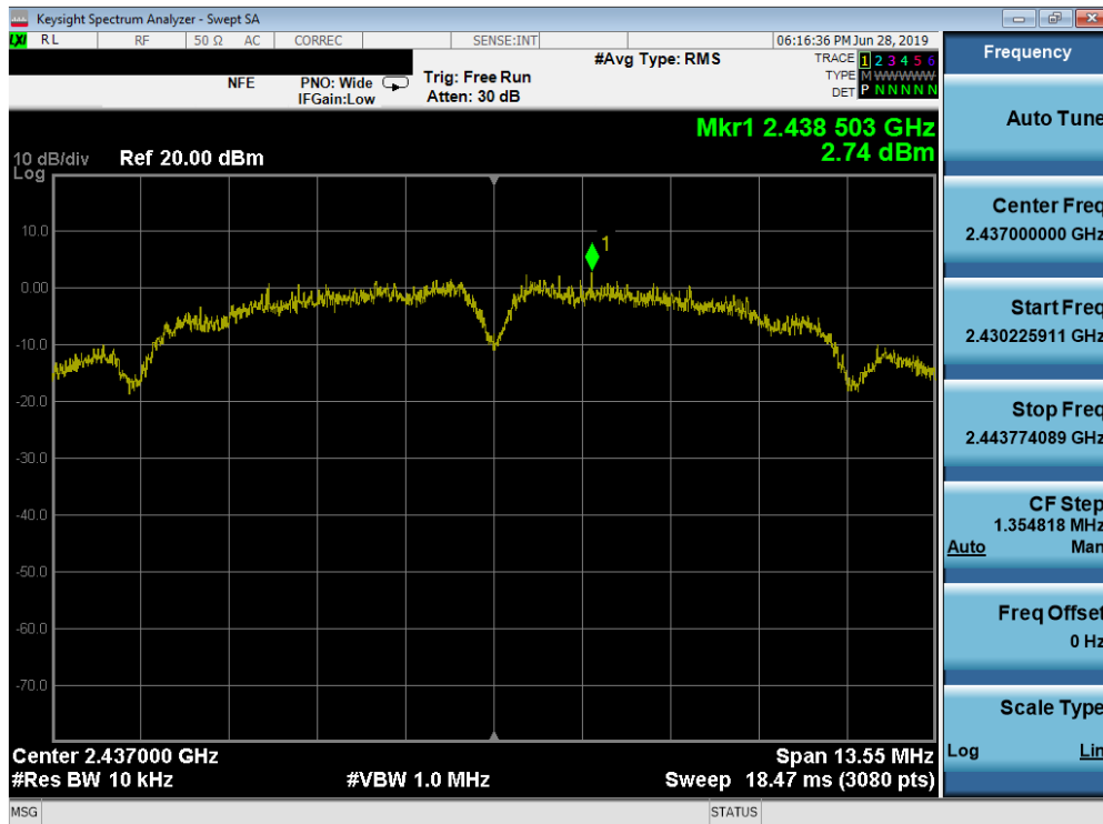
Plot 7-11. Power Spectral Density Plot (802.11b – Ch. 6)
