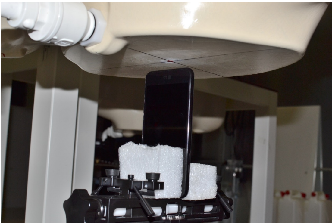
SAR Test Setup Photo 8: Bottom at 1.0 cm
