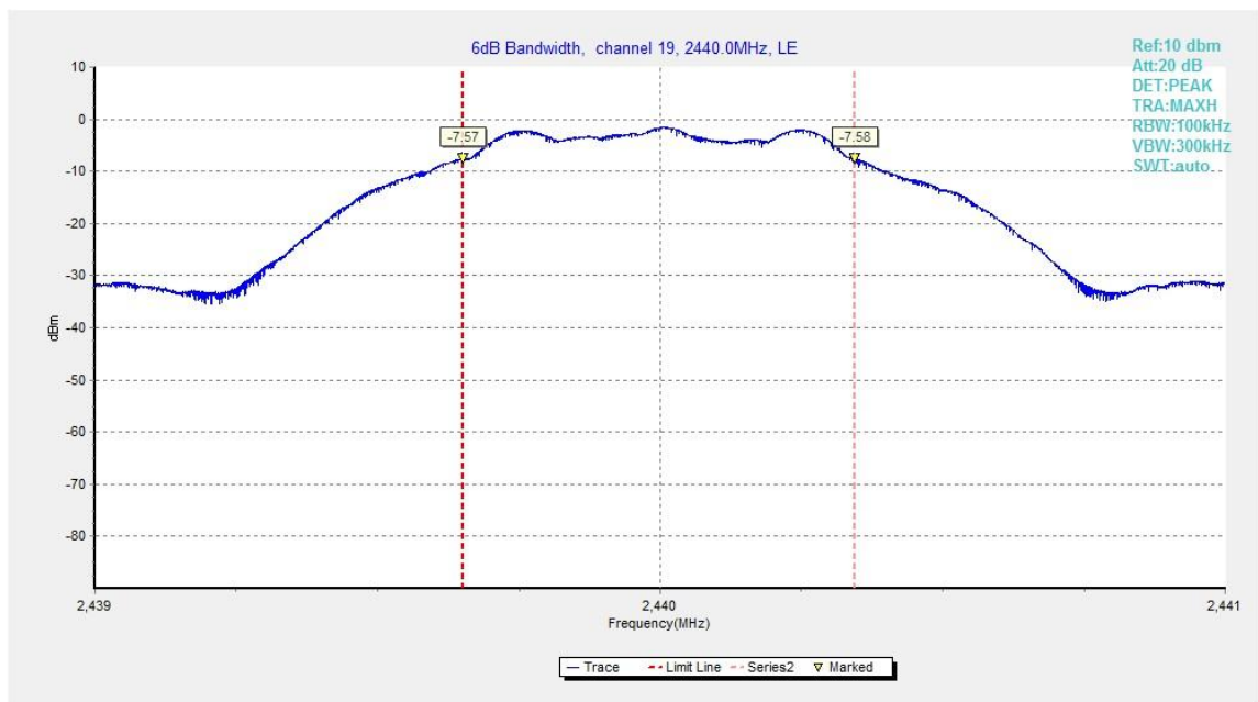
Fig.21. 6dB Bandwidth: GFSK, 2440 MHz
