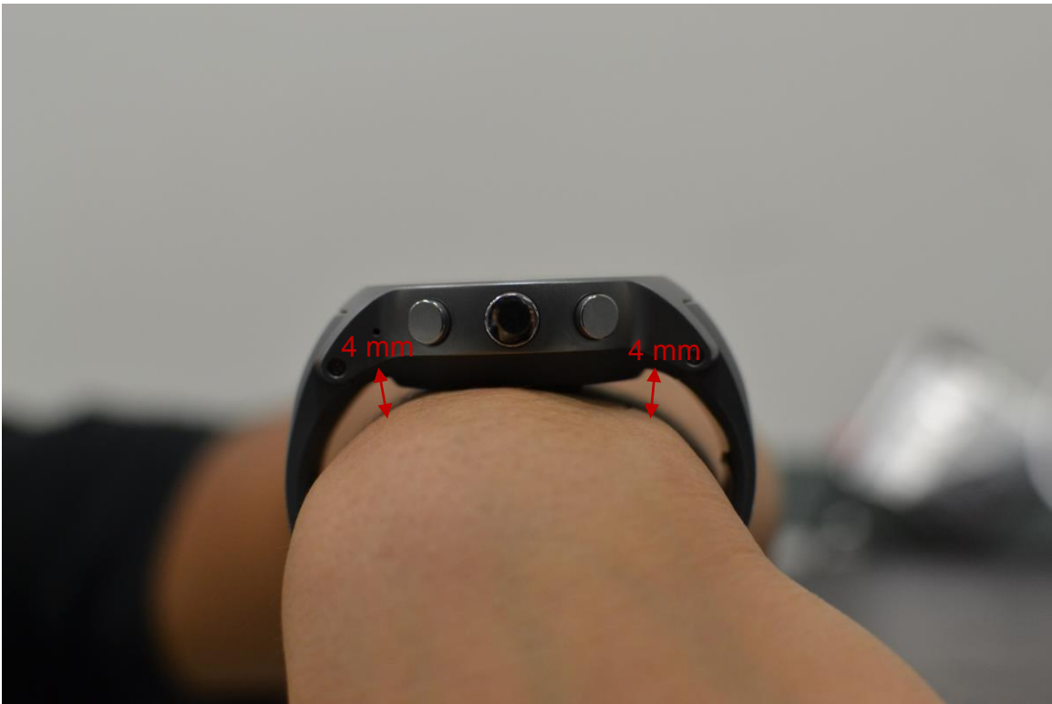
SAR Test Setup Photo 4 – DUT actual use condition with gap at hinge
