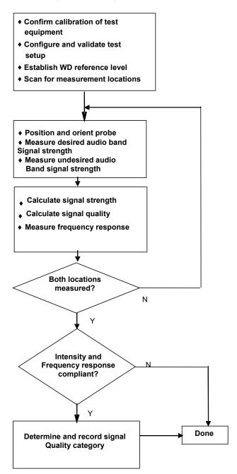
Figure 4-16 C63.19 T-Coil Signal Test Process
