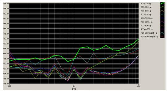
Figure 6-1 **CDMA Audio Band Magnetic Noise**
