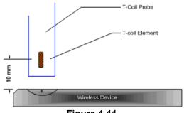
Figure 4-11 Measurement Distance
