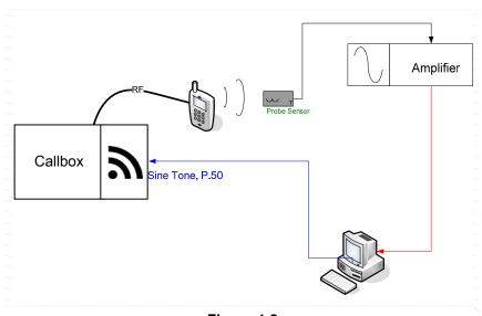
Figure 4-2 T-Coil Test Setup
