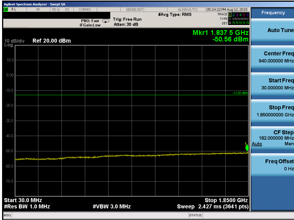
Plot 6-57. Conducted Spurious Plot (PCS WCDMA Mode – Ch. 9400)
