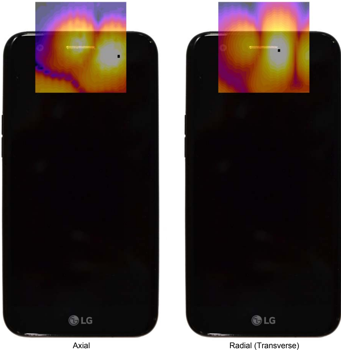
Figure 14-3 T-Coil Scan Overlay Magnetic Field Distributions
