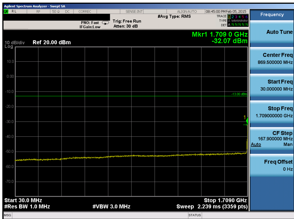
Plot 6-112. Conducted Spurious Plot (Band 4 – 10.0MHz QPSK – RB Size 1, RB Offset 0 – Low Channel)
