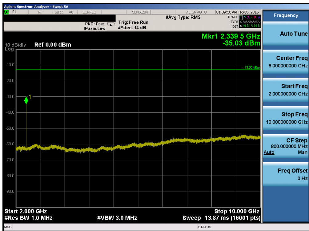
Plot 6-42. Conducted Spurious Plot (Band 13 – 5.0MHz QPSK – RB Size 1, RB Offset 0 – Mid Channel)
