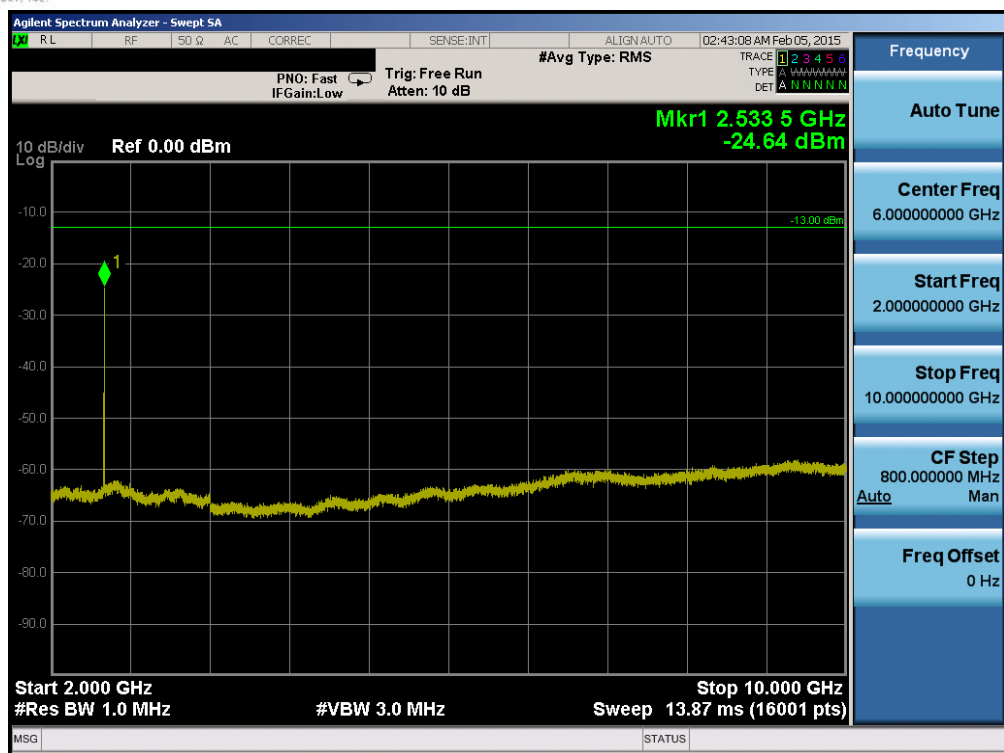
Plot 6-75. Conducted Spurious Plot (Band 5 – 5.0MHz QPSK – RB Size 1, RB Offset 0 – High Channel)
