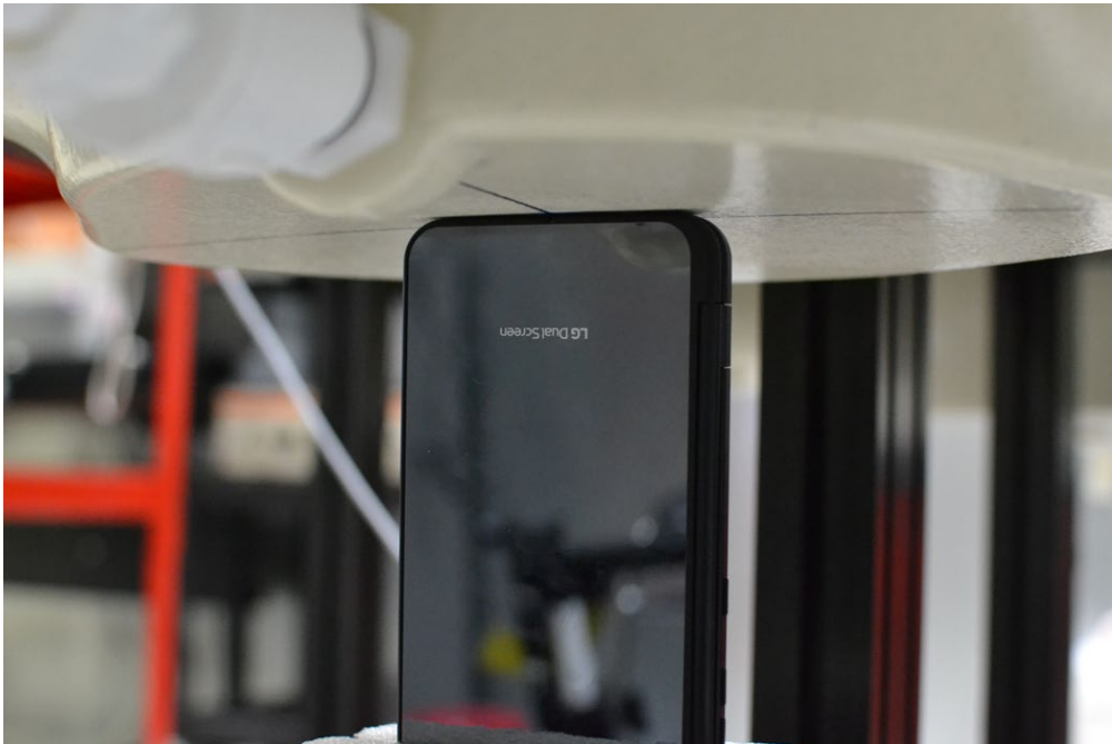
SAR Test Setup Photo 21 – Bottom Side at 0 mm with Dual Display Cover Position #1 (0 degrees)
