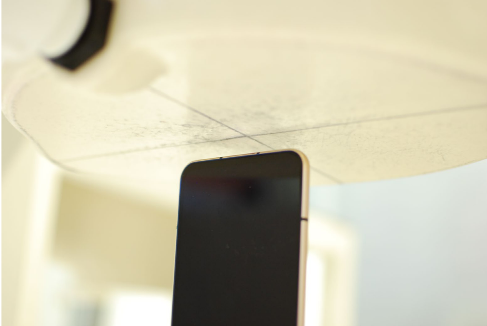
SAR Test Setup Photo 18 – Bottom Edge at 10 mm
