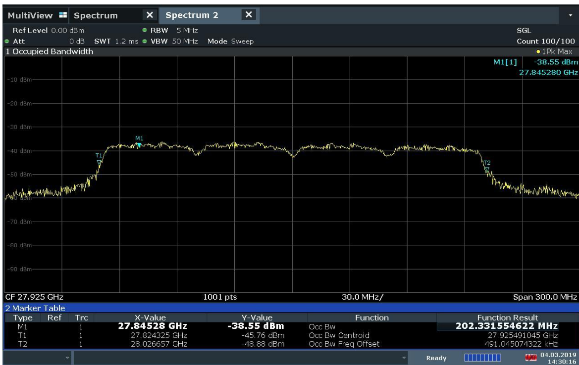
Plot 7-4. Occupied Bandwidth Plot (4CC-50MHz Bandwidth QPSK Mid Channel)
