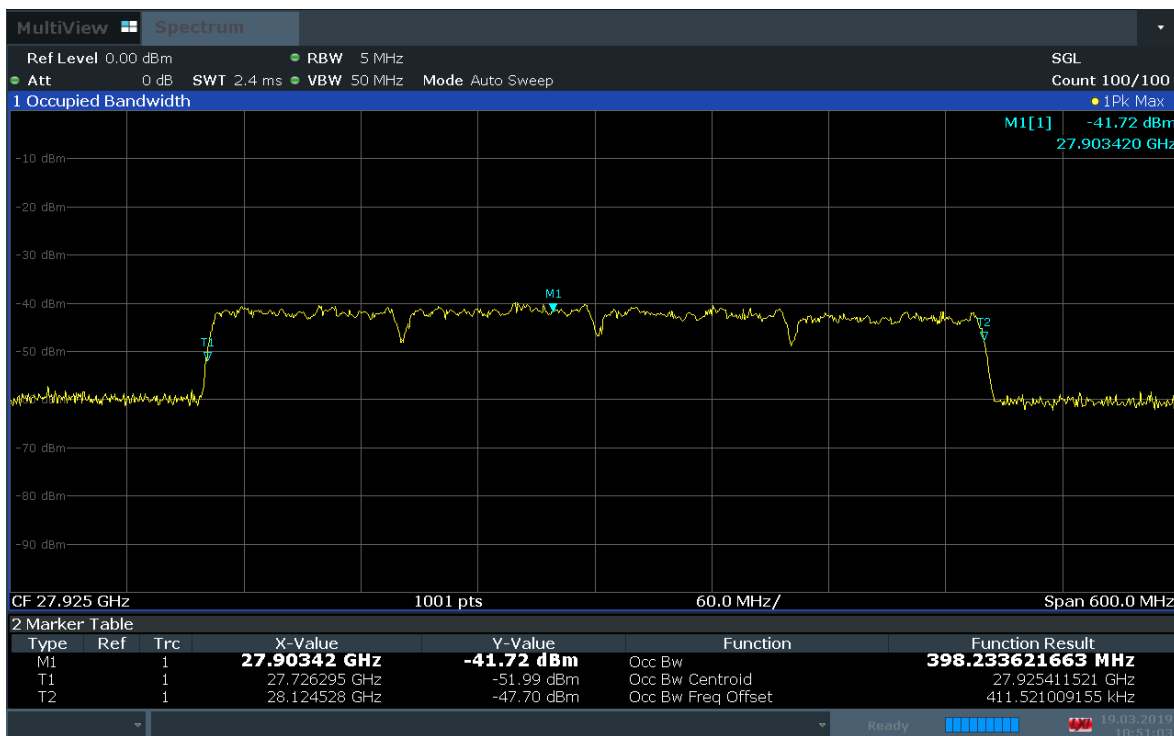
Plot 7-12. Occupied Bandwidth Plot (4CC-100MHz Bandwidth 64QAM Mid Channel)
