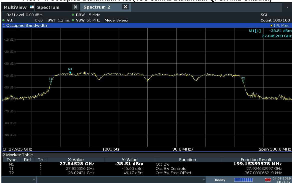
Plot 7-5. Occupied Bandwidth Plot (4CC-50MHz Bandwidth 16QAM Mid Channel)
