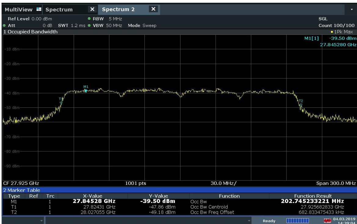
Plot 7-28. Occupied Bandwidth Plot (4CC-50MHz Bandwidth QPSK Mid Channel)
