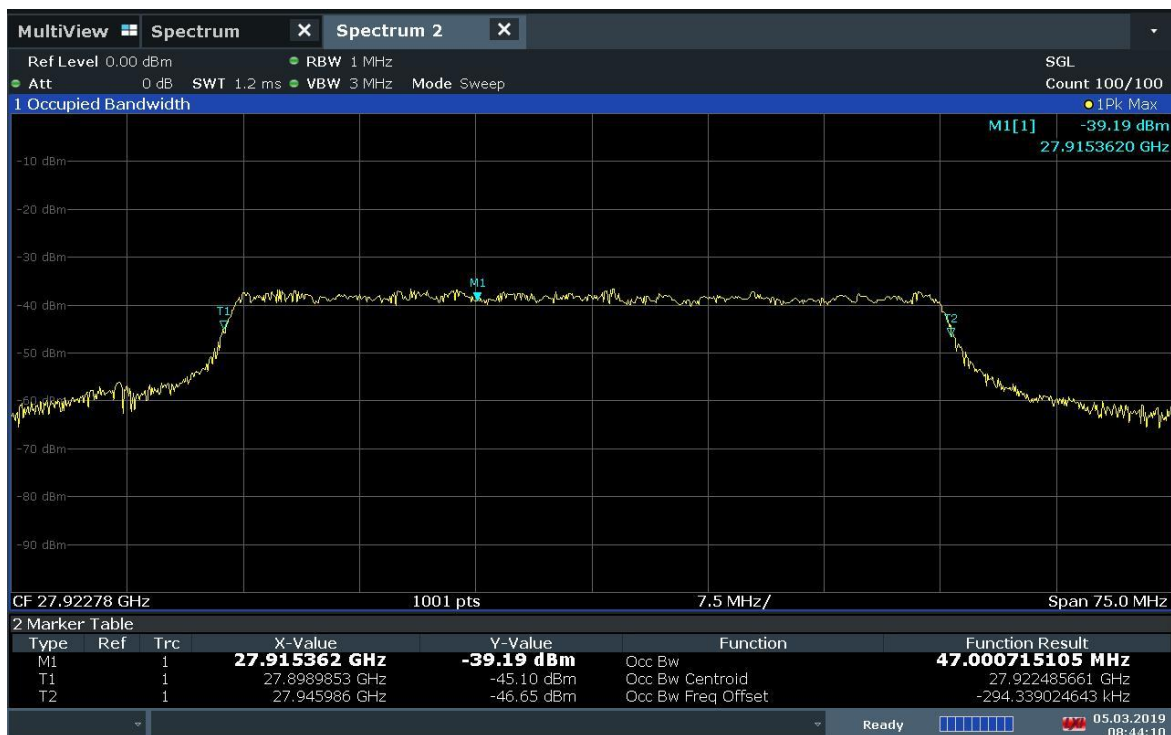
Plot 7-25. Occupied Bandwidth Plot (1CC-50MHz Bandwidth QPSK Mid Channel)
