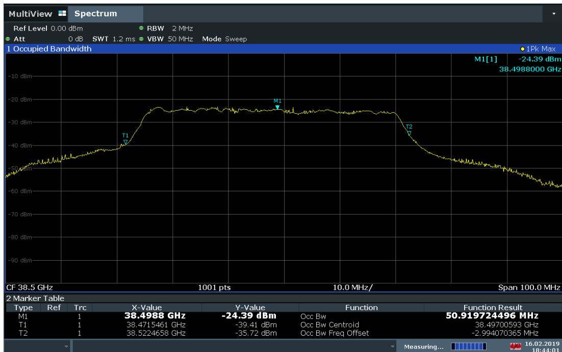
Plot 7-13. Occupied Bandwidth Plot (1CC-50MHz Bandwidth QPSK Mid Channel)
