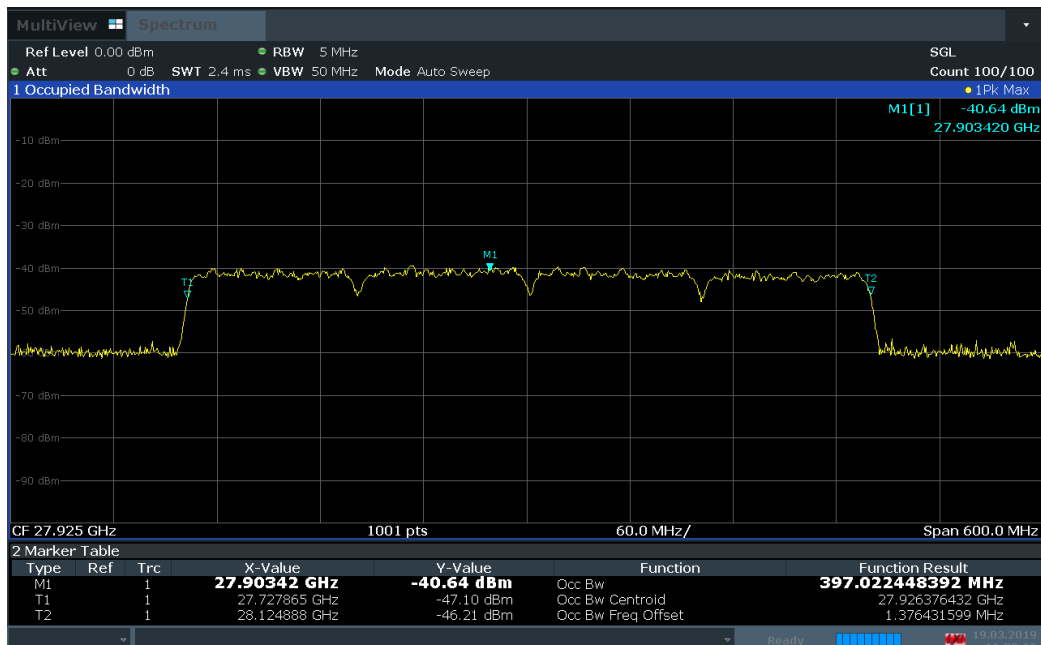
Plot 7-34. Occupied Bandwidth Plot (4CC-100MHz Bandwidth QPSK Mid Channel)
