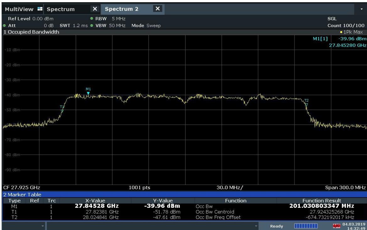
Plot 7-6. Occupied Bandwidth Plot (4CC-50MHz Bandwidth 64QAM Mid Channel)
