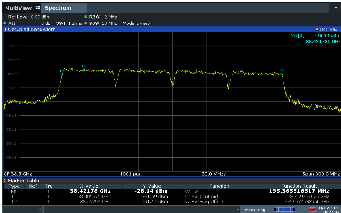
Plot 7-18. Occupied Bandwidth Plot (4CC-50MHz Bandwidth 64QAM Mid Channel)
