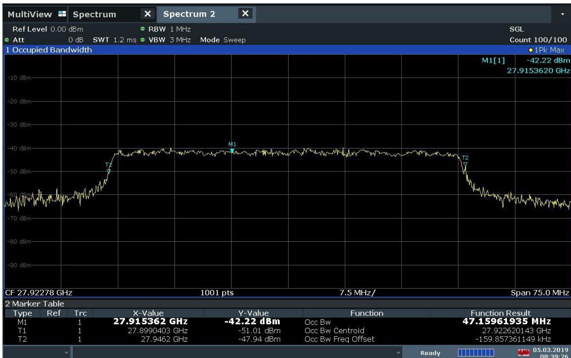
Plot 7-3. Occupied Bandwidth Plot (1CC-50MHz Bandwidth 64QAM Mid Channel)
