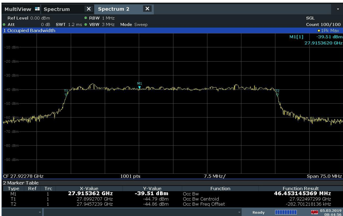
Plot 7-26. Occupied Bandwidth Plot (1CC-50MHz Bandwidth 16QAM Mid Channel)
