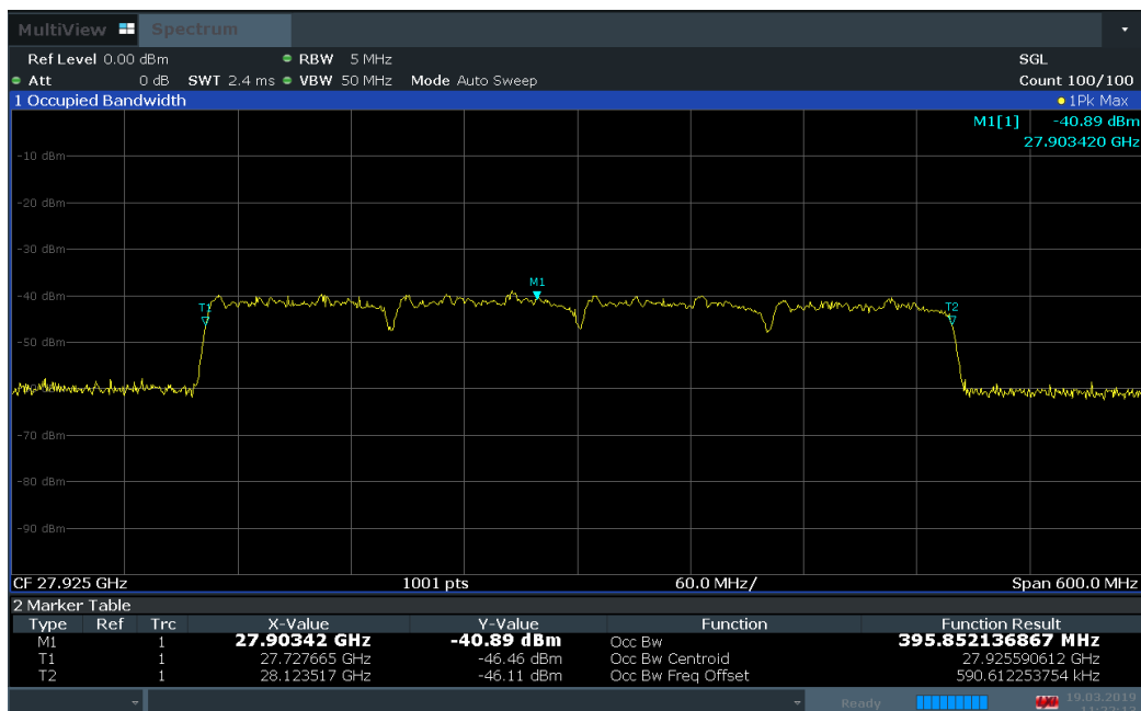
Plot 7-36. Occupied Bandwidth Plot (4CC-100MHz Bandwidth 64QAM Mid Channel)
