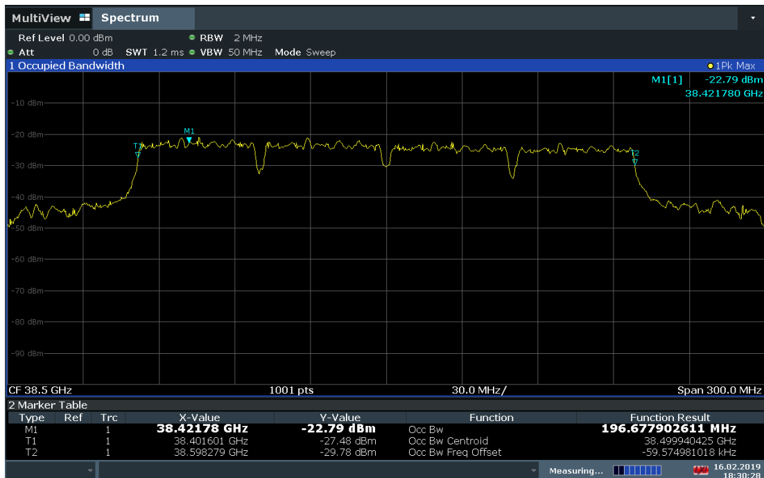
Plot 7-40. Occupied Bandwidth Plot (4CC-50MHz Bandwidth QPSK Mid Channel)
