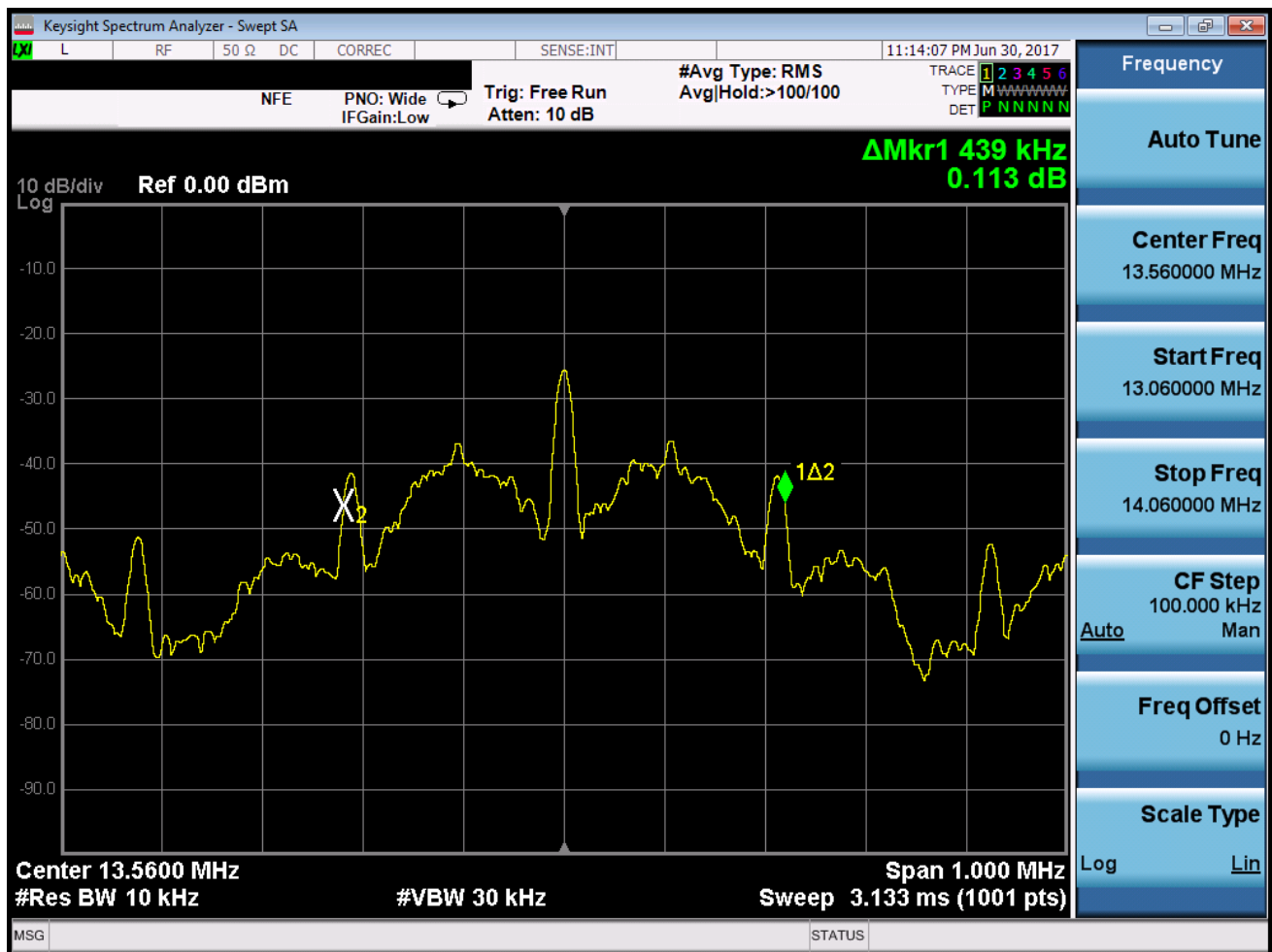
Figure 7-2. 20dB Bandwidth Plot
