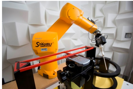
Figure 4-3 SPEAG Robotic System
