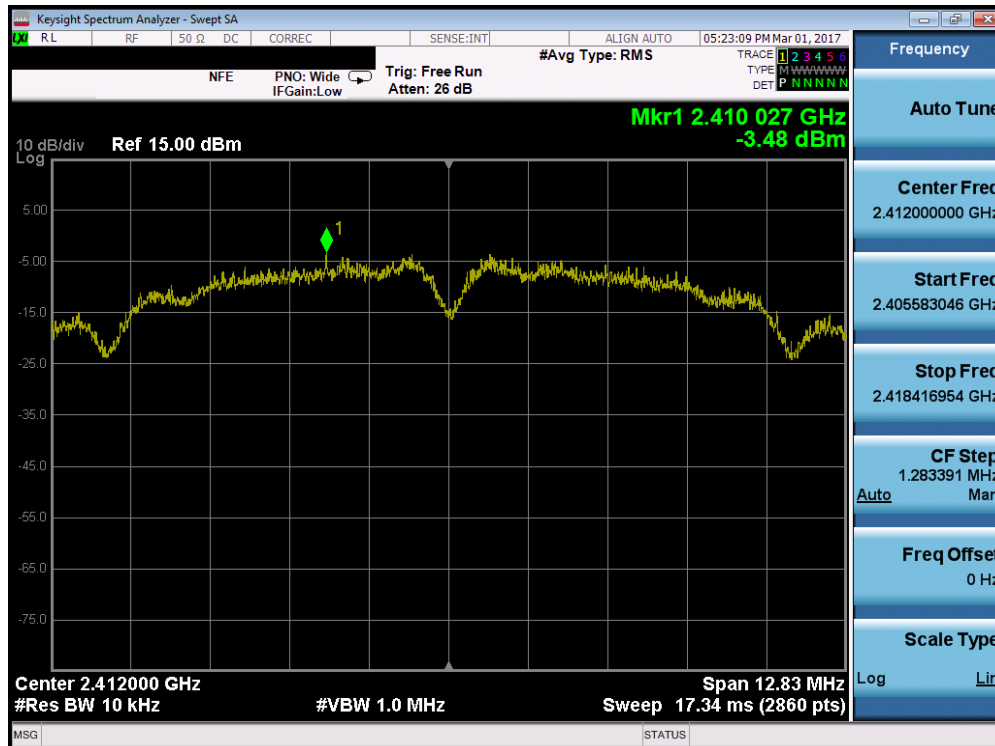
Plot 7-10. Power Spectral Density Plot (802.11b – Ch. 1)
