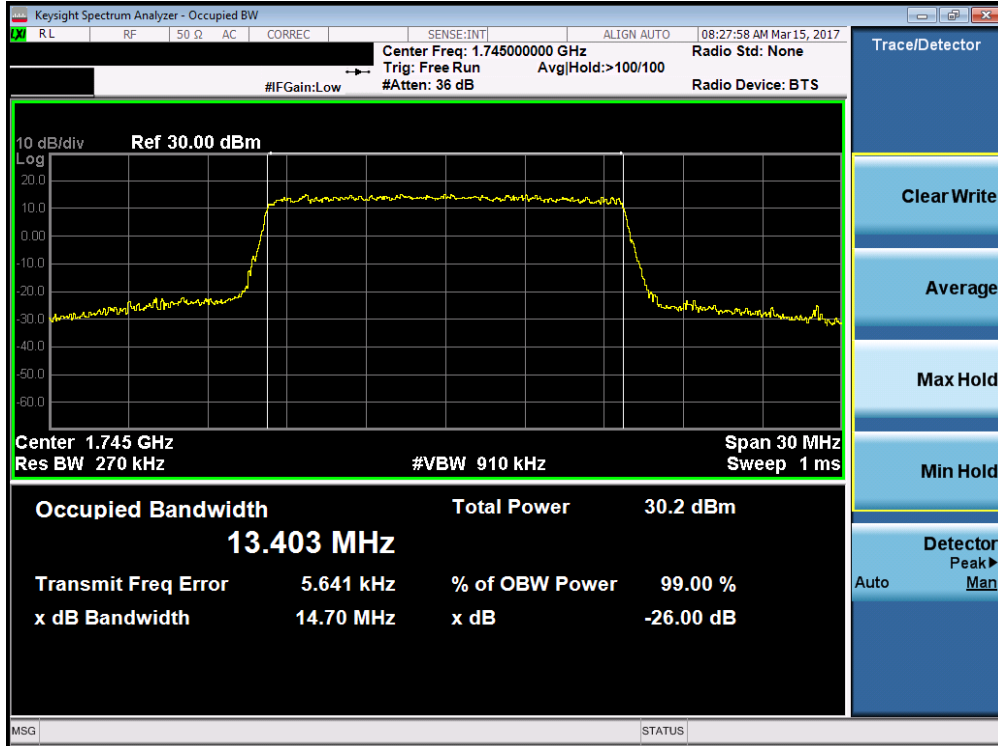
Plot 7-39. Occupied Bandwidth Plot (Band 4/66 – 15.0MHz 64-QAM – RB Size 75)
