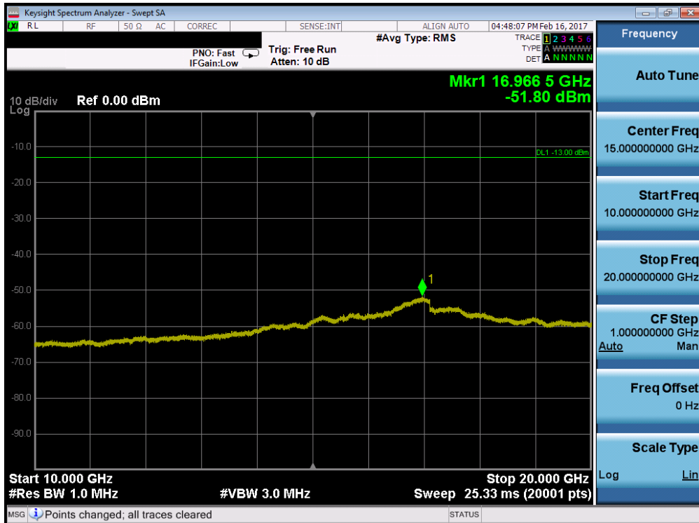
Plot 7-102. Conducted Spurious Plot (Band 2 – 10.0MHz QPSK – RB Size 1, RB Offset 0 – Low Channel)
