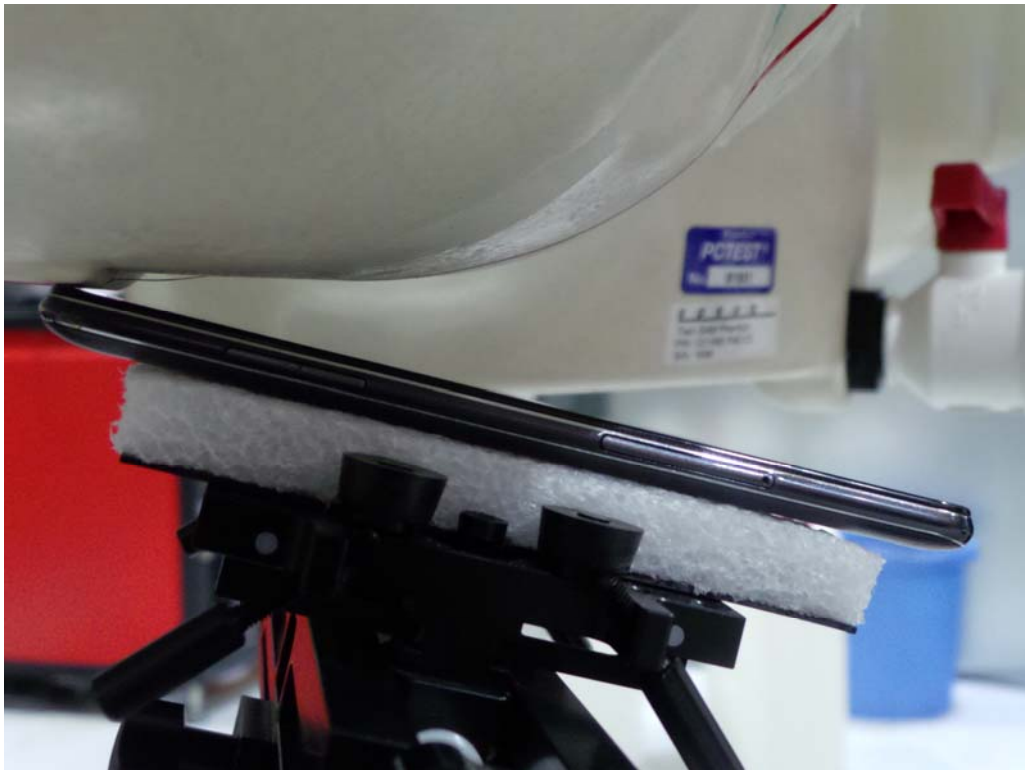
SAR Test Setup Photo 2: Right Tilt
