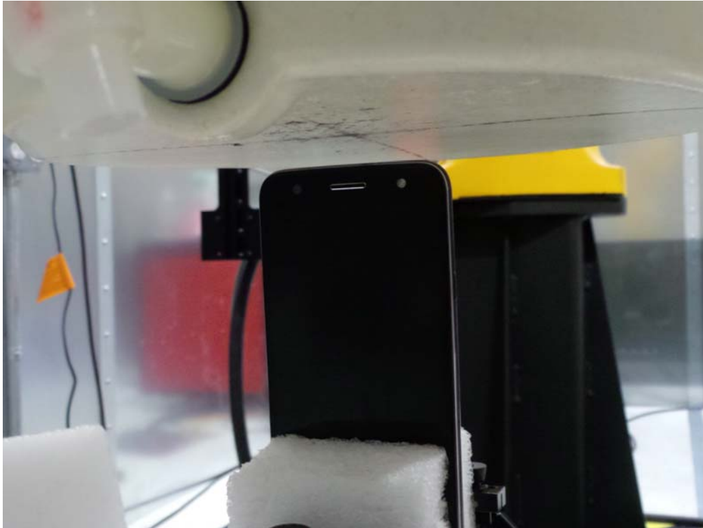
SAR Test Setup Photo 7: Top Edge at 10 mm
