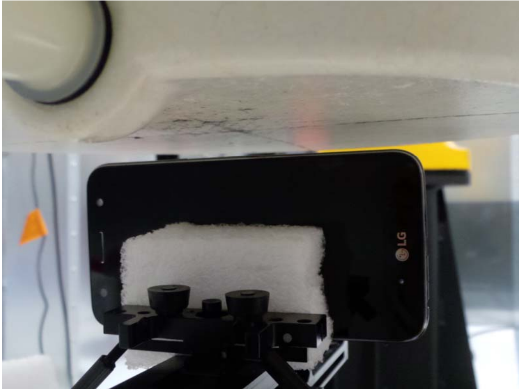
SAR Test Setup Photo 9: Right Edge at 10 mm
