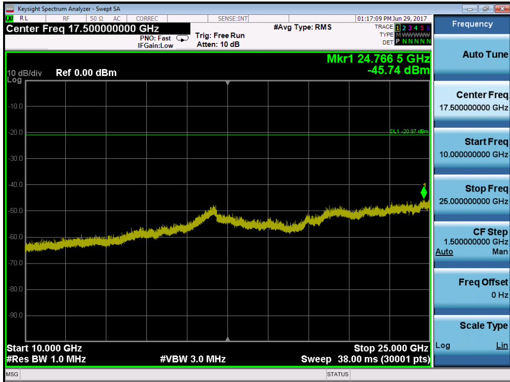
Plot 7-17. Conducted Spurious Plot (Bluetooth (LE), 1Mbps – Ch. 39)
