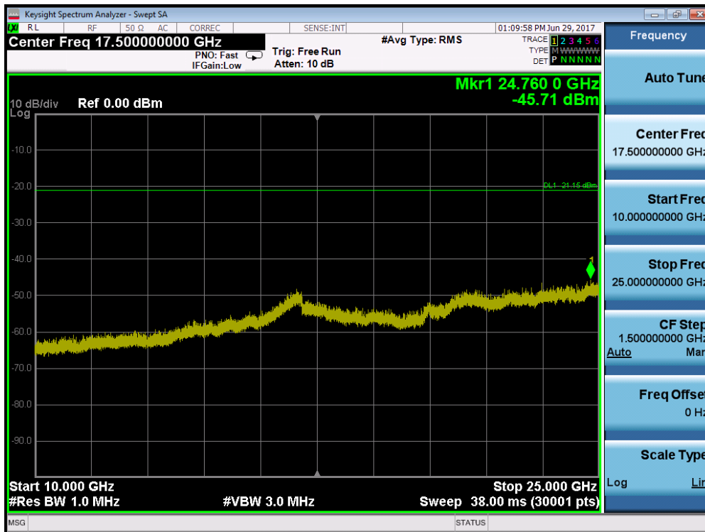
Plot 7-13. Conducted Spurious Plot (Bluetooth (LE), 1Mbps – Ch. 0)
