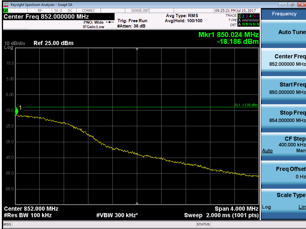
Plot 7-132. Upper Extended Band Edge Plot (Band 5/26 – Band 5 – 3.0MHz QPSK – RB Size 15)
