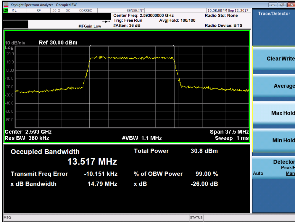
Plot 7-53. Occupied Bandwidth Plot (Band 41 - 15.0MHz QPSK - Full RB Configuration)
