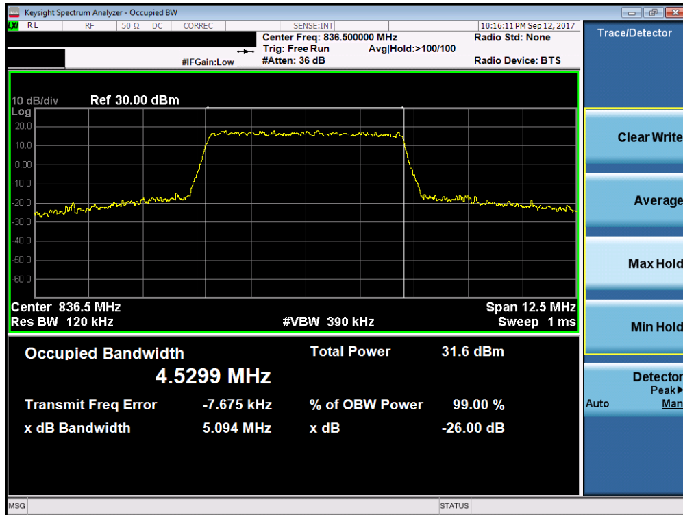
Plot 7-19. Occupied Bandwidth Plot (Band 26/5 - 5.0MHz QPSK - Full RB Configuration)
