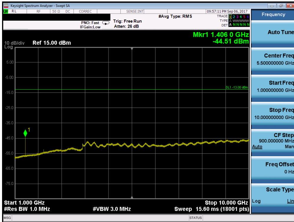
Plot 7-62. Conducted Spurious Plot (Band 12 - 10.0MHz QPSK - RB Size 1, RB Offset 0 - Mid Channel)
