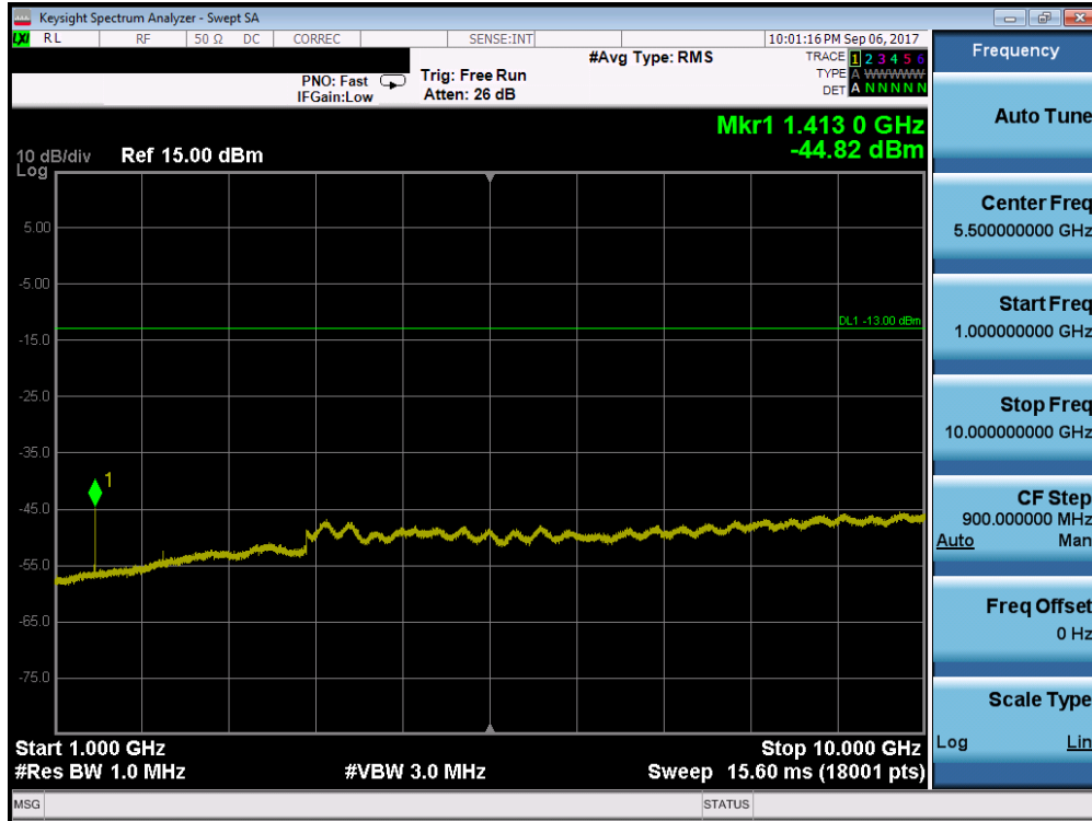
Plot 7-65. Conducted Spurious Plot (Band 12 - 10.0MHz QPSK - RB Size 1, RB Offset 0 - High Channel)
