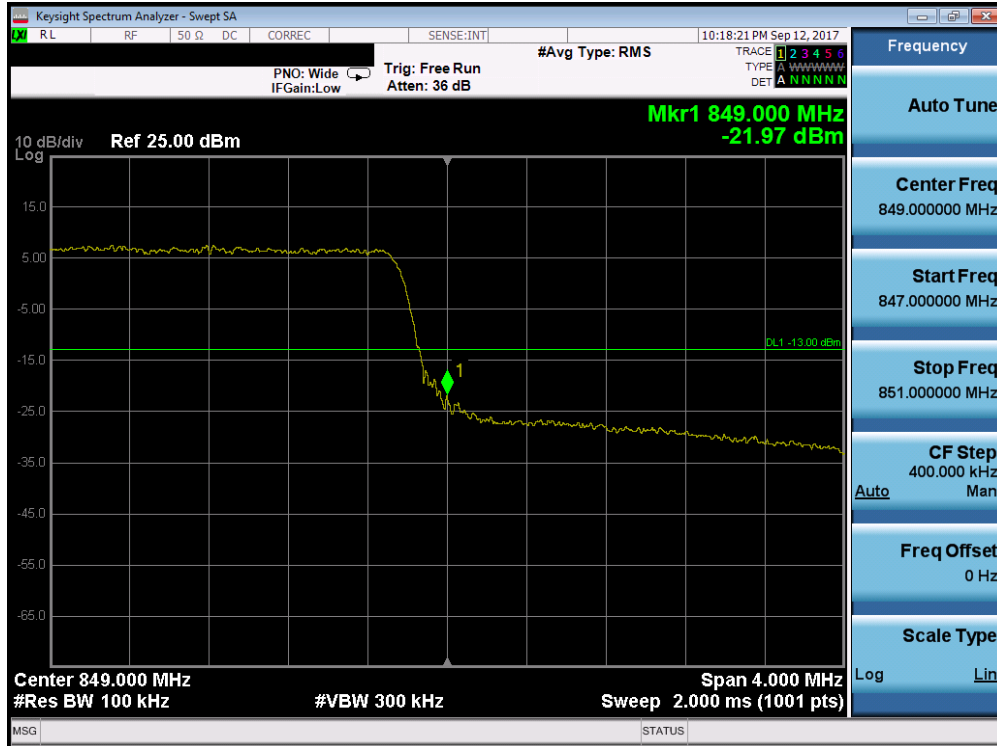
Plot 7-122. Upper Band Edge Plot (Band 26/5 - 5.0MHz QPSK - Full RB Configuration)
