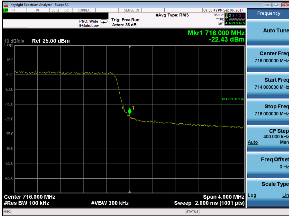
Plot 7-110. Upper Band Edge Plot (Band 12 - 5.0MHz QPSK - Full RB Configuration)
