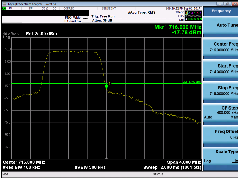
Plot 7-106. Upper Band Edge Plot (Band 12 - 1.4.0MHz QPSK - Full RB Configuration)
