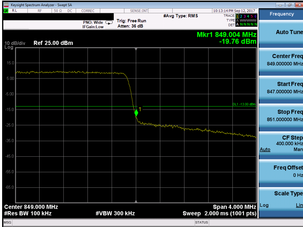
Plot 7-120. Upper Band Edge Plot (Band 26/5 - 3.0MHz QPSK - Full RB Configuration)
