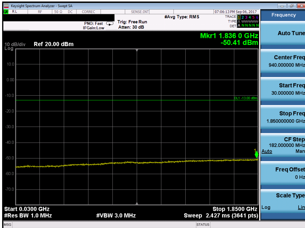
Plot 7-90. Conducted Spurious Plot (Band 25/2 - 5.0MHz QPSK - RB Size 1, RB Offset 0 - Mid Channel)
