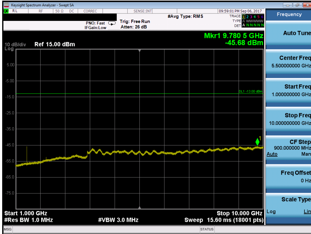
Plot 7-59. Conducted Spurious Plot (Band 12 - 10.0MHz QPSK - RB Size 1, RB Offset 0 - Low Channel)
