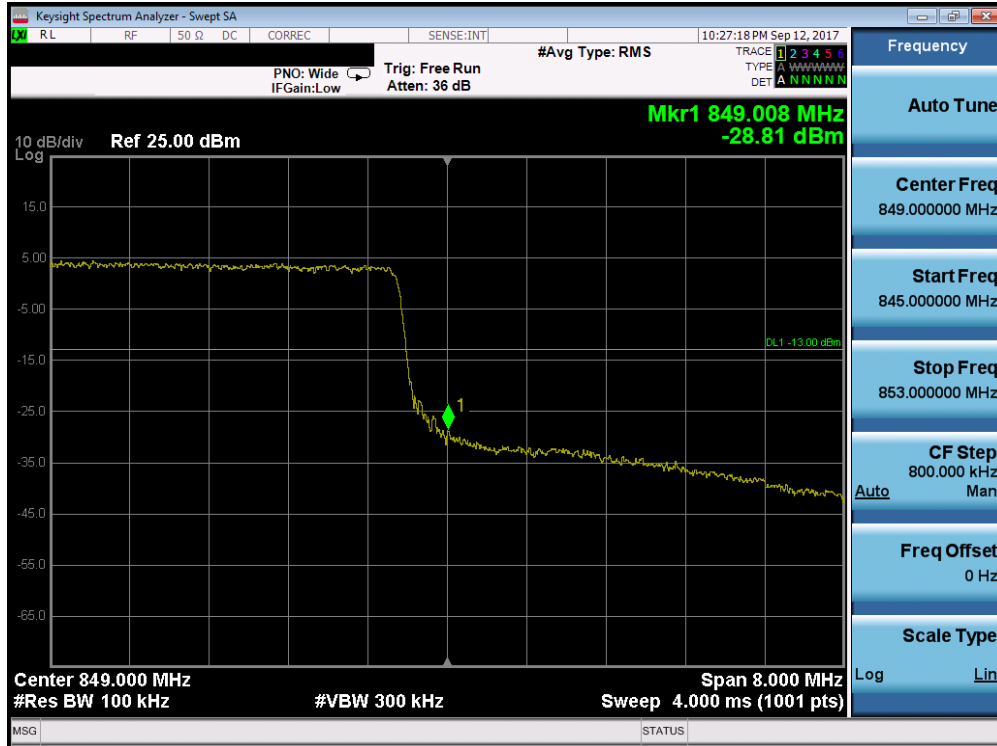
Plot 7-124. Upper Band Edge Plot (Band 26/5 - 10.0MHz QPSK - Full RB Configuration)
