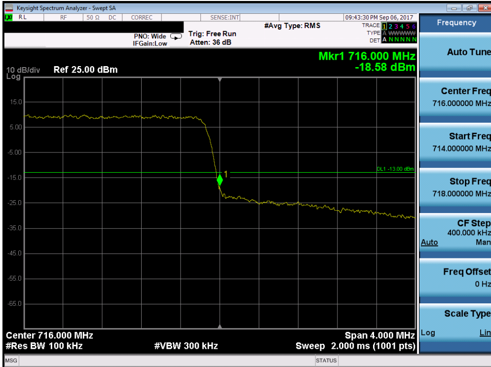
Plot 7-108. Upper Band Edge Plot (Band 12 - 3.0MHz QPSK - Full RB Configuration)
