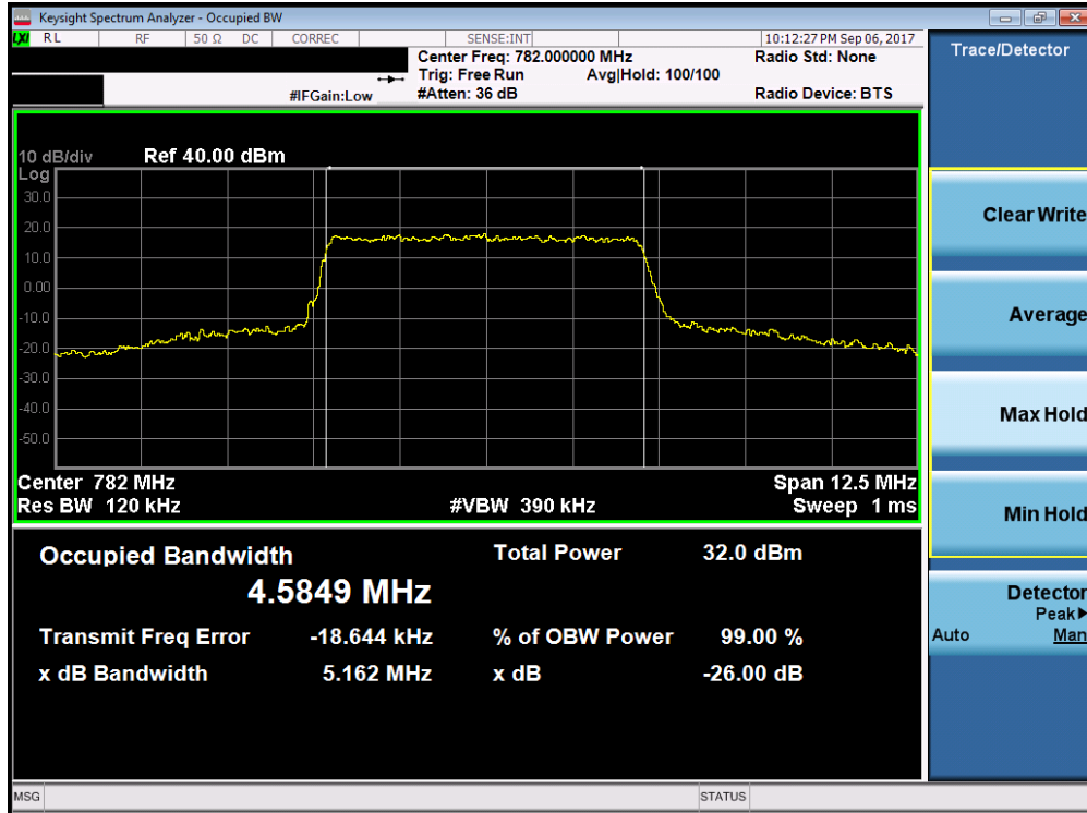
Plot 7-11. Occupied Bandwidth Plot (Band 13 - 5.0MHz QPSK - Full RB Configuration)
