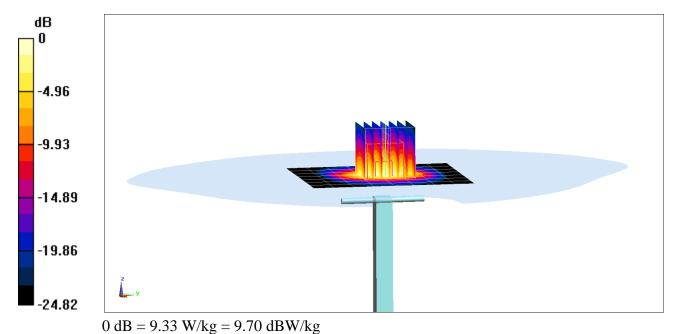
DUT: Dipole 750 MHz; Type: D750V3; Serial: 1054
