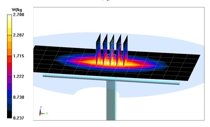
DUT: Dipole 1750 MHz; Type: D1750V2; Serial: 1148
