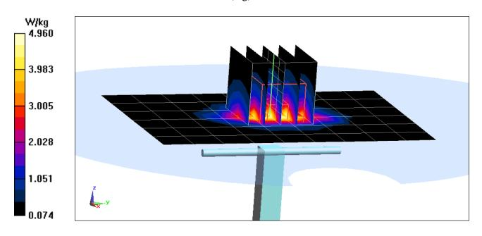
DUT: Dipole 2450 MHz; Type: D2450V2; Serial: 719
